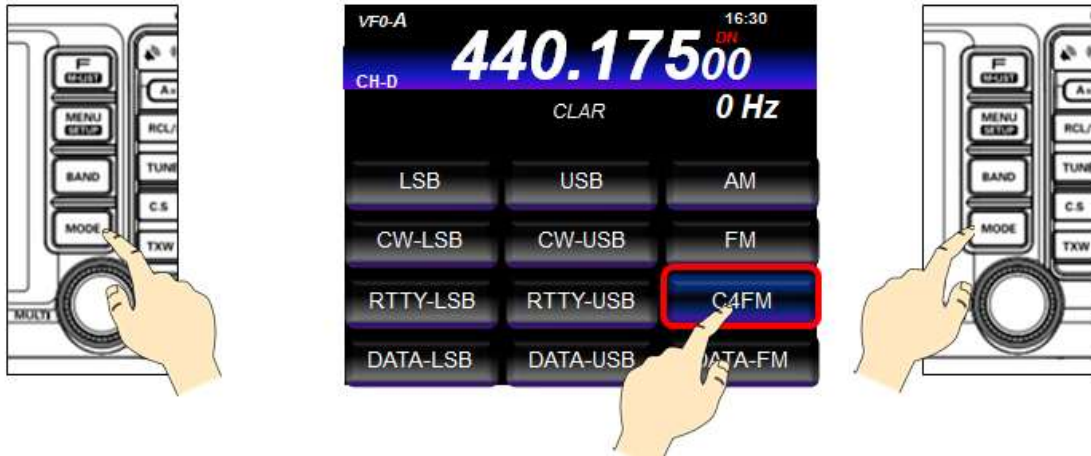
Figure 70 press MODE button, touch “C4FM”, then the MODE Button again
