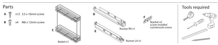
Fit runners to cabinet sides. We recommend this operation is carried out before cabinet carcass is assembled.
