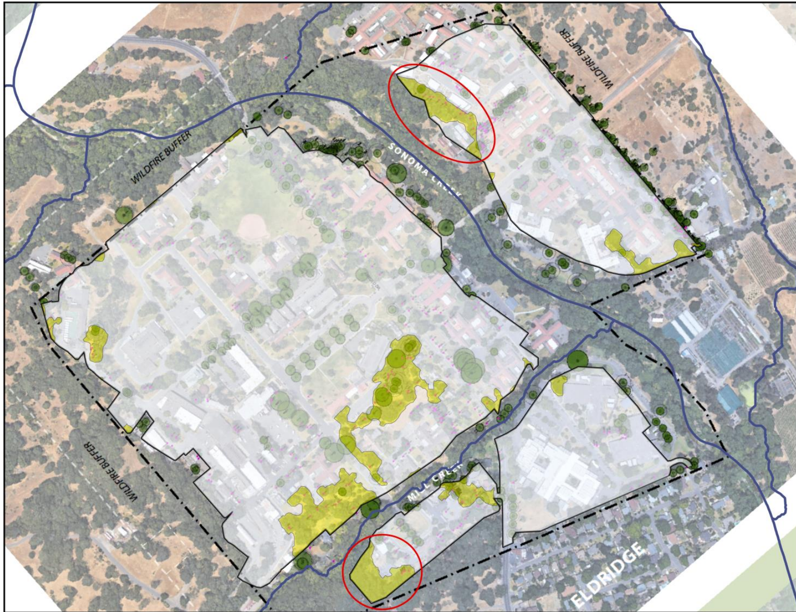
Figure 4. Map shows Project Grading Limits from the Vesting Tentative Map (white areas) as compared to sensitive vegetation types (yellow), overlaid on the Project Arborist report. Red circles indicate areas where grading / fill (i.e. forest removal) is proposed, but not addressed in the Arborist report. The Arborist report was prepared to fulfill Sonoma County ordinances around the removal of sensitive tree species, but does not “mitigate” for the environmental impacts of removing sensitive vegetation types, or the impacts of urban forest removal on native wildlife species.
