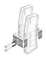
When assembling the coupler, position the magazine on the left higher than the magazine on the right. Magazines like PMAGS will fit into place on the notches of the coupler front plate. This offset will prevent you from possibly blocking the ejection port from spent casings.
