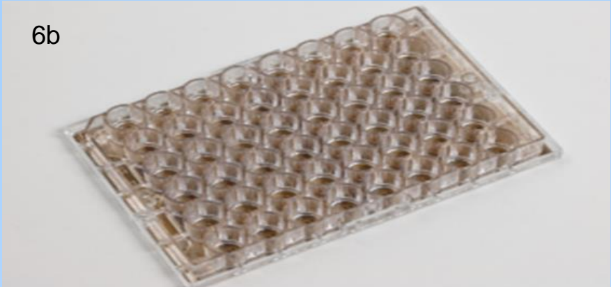
Figure 6b: 48 Well MEA • Higher throughput 48-well configuration • 16 low-noise microelectrodes per well • 4 integrated ground electrodes per well • Polymer (Kapton) insulation • Nano-textured Gold electrodes • ANSI compliant well plates • Evaporation-reducing lid
