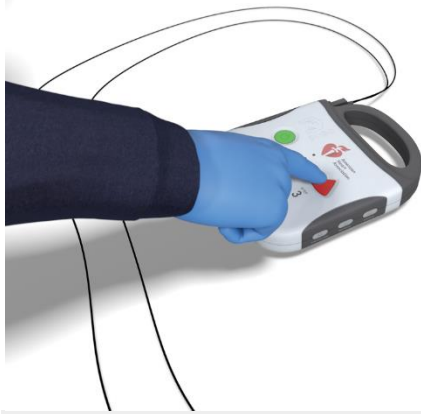
Figure 23B. When everyone is clear of the person, the AED operator presses the Shock button.
