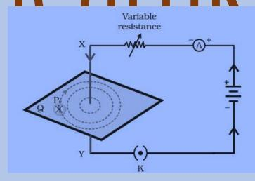
the deflection of the compass needle placed at a given point if the current in the copper wire is changed
