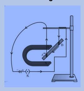
The displacement of the rod in the above activity suggests that a force is exerted on the current-carrying aluminium rod when it is placed in a magnetic field. It also suggests that the direction of force is also reversed when the direction of current through the conductor is reversed.
