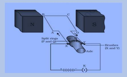
When the axle attached to the two rings is rotated such that the arm AB moves up (and the arm CD moves down) in the magnetic field produced by the permanent magnet.
