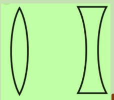
A convex lens converges (bends inward) the light generally falling on it. Therefore, it is called a converging lens. On the other hand, a concave lens diverges (bends outward) the light and is called a diverging lens.
