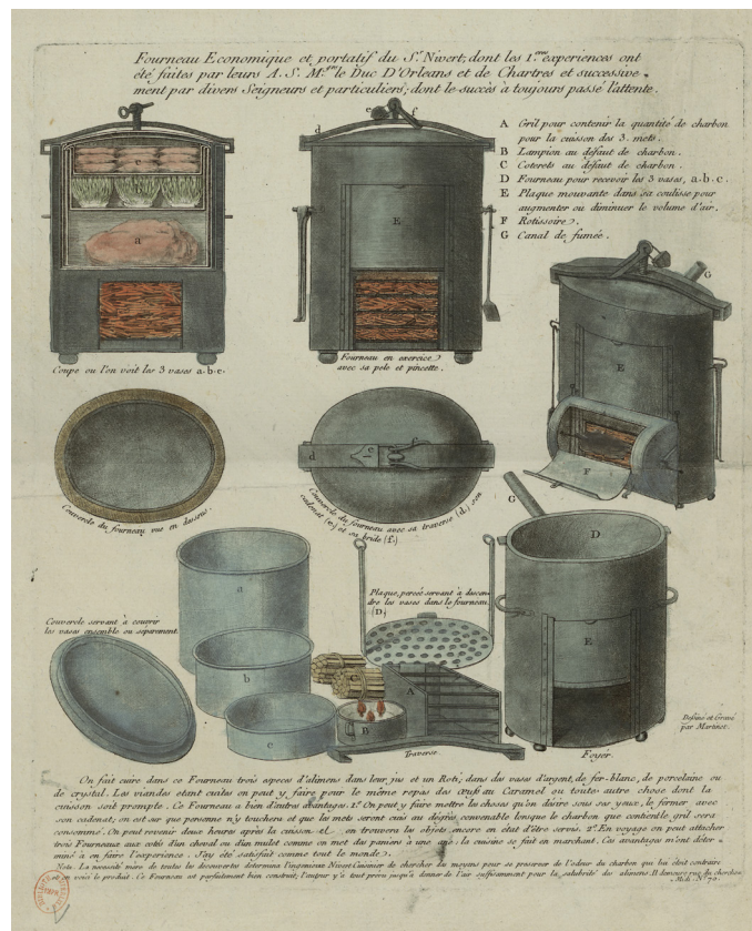
Figure 24. Frenchman Louis Nivert’s 1780 Nouveaux fourneaux économiques et portatifs (“New economical and portable furnace”), a portable cooking apparatus, or “portable kitchen.”
