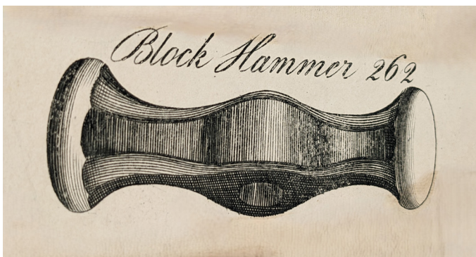
Figure 6. Block hammer, used for doming and raising tinplate.
