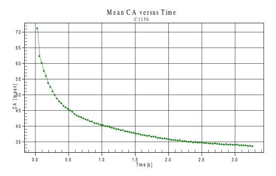
Capstone 1150 fluoro surfactant note the exponential decay in contact angle i.e. wetting is slowing down and will never reach zero degrees
