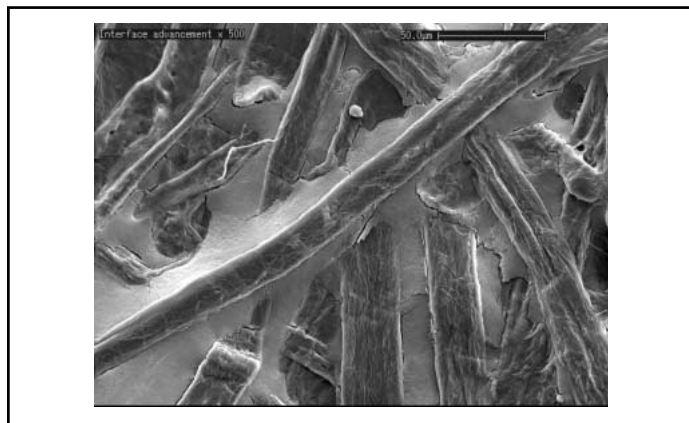
Fig. 3. The typical fluid distribution in the midst of the saturated zone. One observes that pores at the surface are not all filled and fibres at depth are still visible to the surface.
