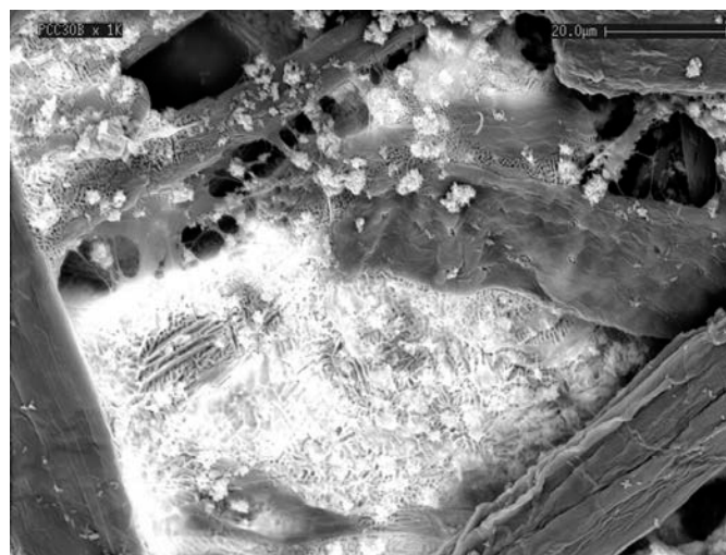
Figure 7.42: Higher magnification image of a 30% PCC filled paper showing more detail of imbibition of clumps of particles.
