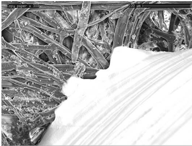
Figure 6.26: SEM secondary electron image of fluid droplet frozen 30 seconds after placement onto sized copy paper.
