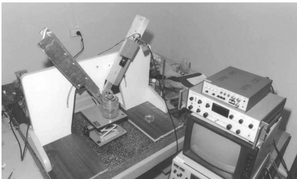
Figure 4.3: Experimental set-up for relative reflectance measurements
