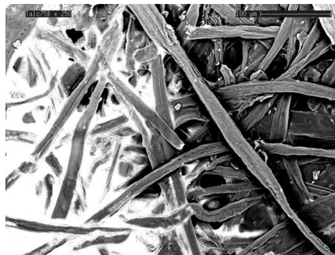
Figure 7.28: Higher magnification image of a 7.5% talc filled paper showing more detail of pore filling.
