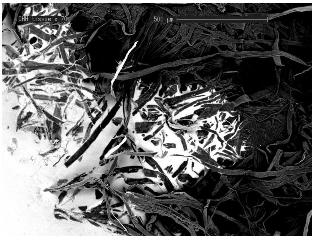
Cryo-SEM image of fluid imbibing into tissue paper.
