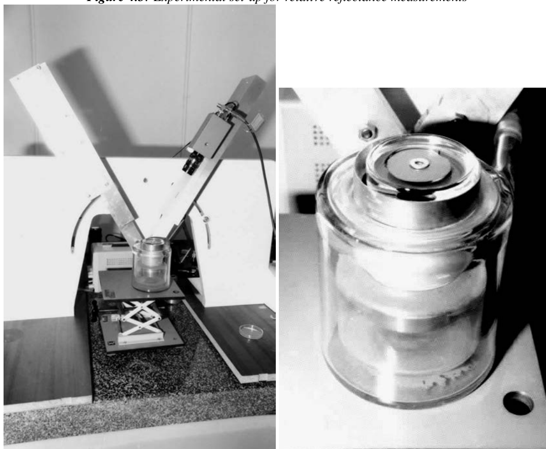
Figure 4.3: Experimental set-up for relative reflectance measurements
