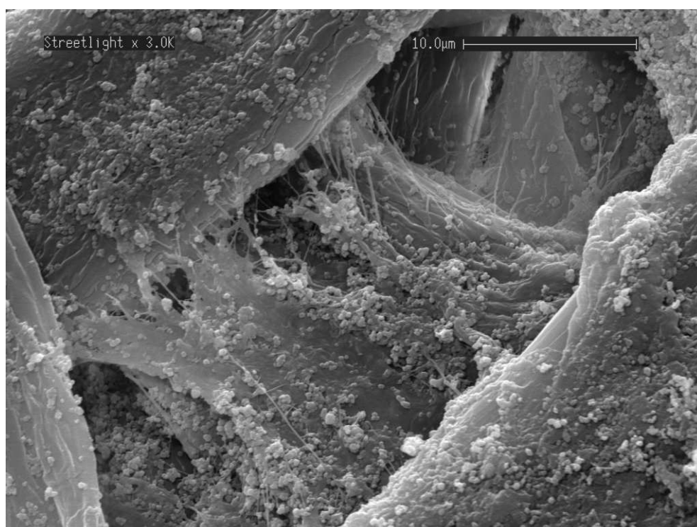
Figure 8.17: High magnification SEM images of unresinated Streetlight showing filler particles, which appear heterogeneously distributed.
