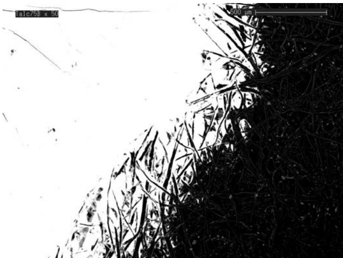
Figure 7.27: Low magnification image of wetting of paper filled with 7.5% talc. Note unfilled pores in comparison to Figure 7.23. Arrows show unfilled pores behind wetting front.
