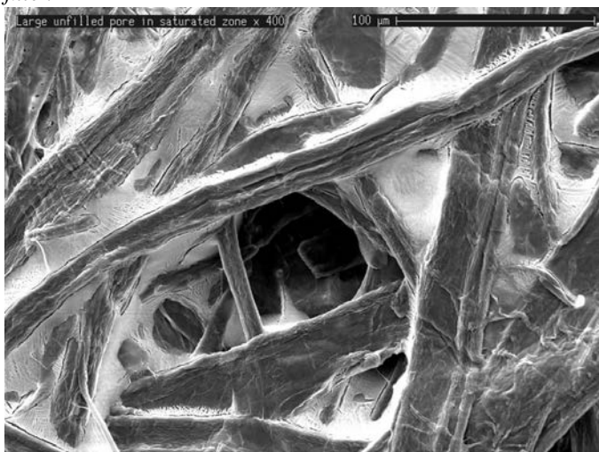
Figure 7.19: Low magnification image of wetting of a paper with no filler.
