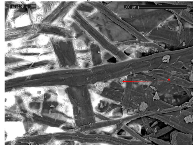
Figure 7.36: Higher magnification image of a 15% talc filled paper showing more detail wetting.
