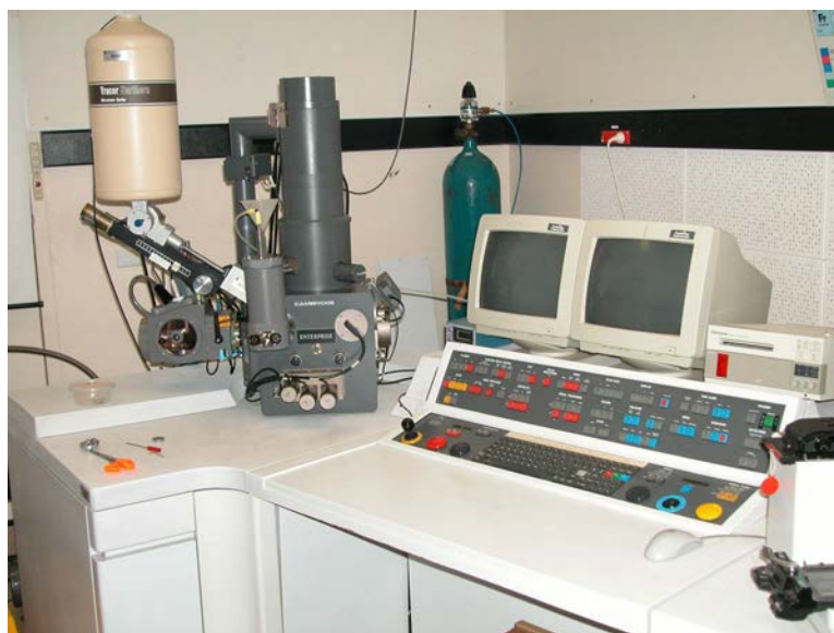
Figure 3.4: Cambridge Instruments S360 Stereoscan scanning electron microscope
