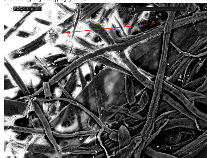
Figure 7.24: Higher magnification image of a 7.5% PCC filled paper showing infilling of pores.
