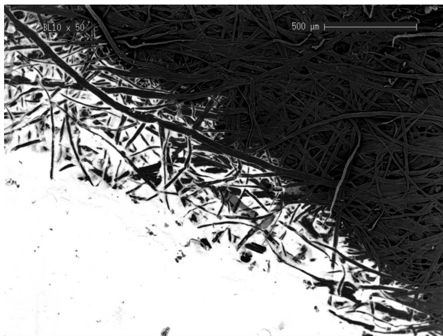
Figure 7.8: Low magnification image of wetting of an unfilled plasma treated paper. Note that there are fewer unfilled pores than in untreated papers (Figure 7.19).
