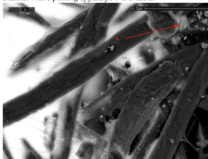
Figure 7.32: Higher magnification image of a 15% PCC filled paper showing film flow at edge of wetting area. Arrow A shows particles of PCC being readily wet and arrow B shows particles in a fibre overlap channel where pinning of fluid flow is evident.
