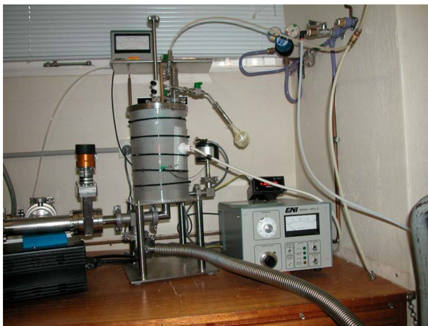
Figure 7.3: Plasma reactor setup including chamber and RF generator
