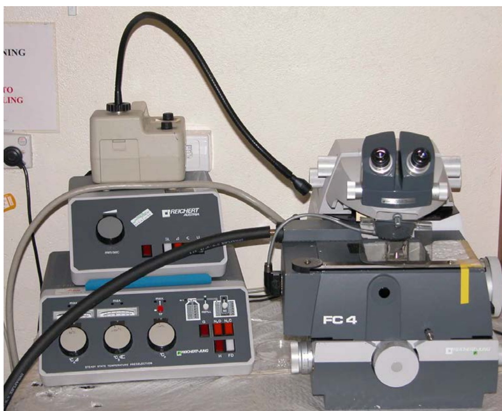
Figure 6.7: Reichert Jung FC4 Ultracut cryo-microtome.
