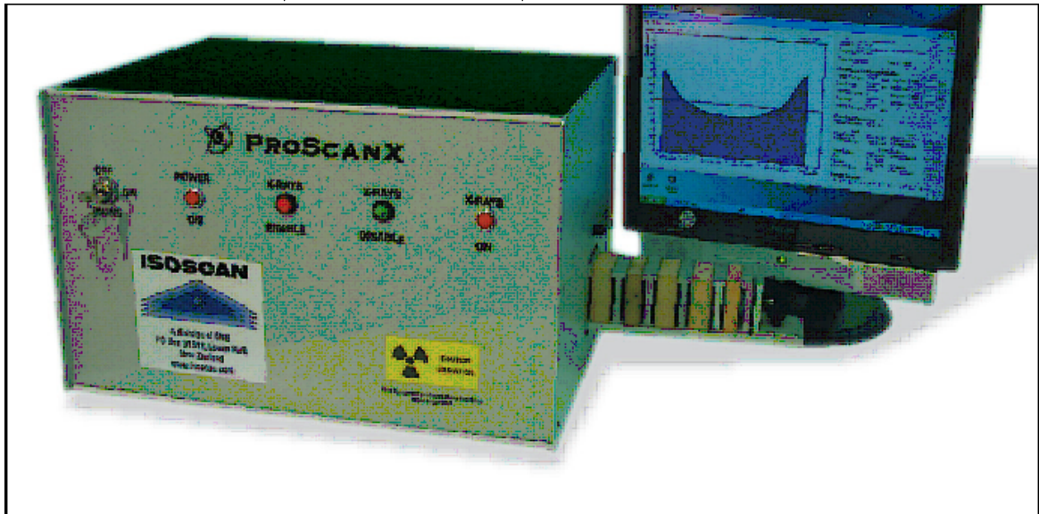
Figure 4. An X-ray sourced density scanner used to determine through panel density
