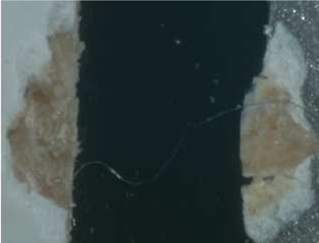
Figure 7. Light microscopy image x16 showing both the void and particle caused by chipout. Note that the evidence of sapstain in the hole is not evident in the removed particle, i.e. the particles which were removed were whole and not fractured.
