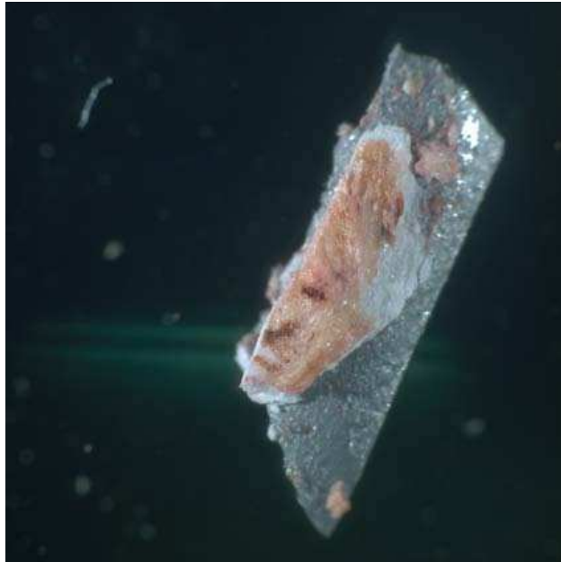
Figure 13. Light microscopy image x10 showing both particle removed as a result of chip-out, note presence of red dye indicating little resin.
