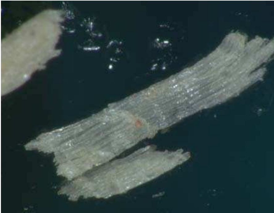
Figure 9. Light microscopy image x32 showing both particle geometry of Gympie surface flake. Note the high surface area to volume (aspect) ratio.
