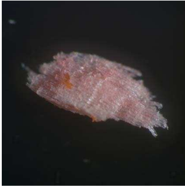
Figure 14. Light microscopy image x20 of blended surface flake ex the G1 spreaders showing little resination as seen by presence of red dye indicating little resin.
