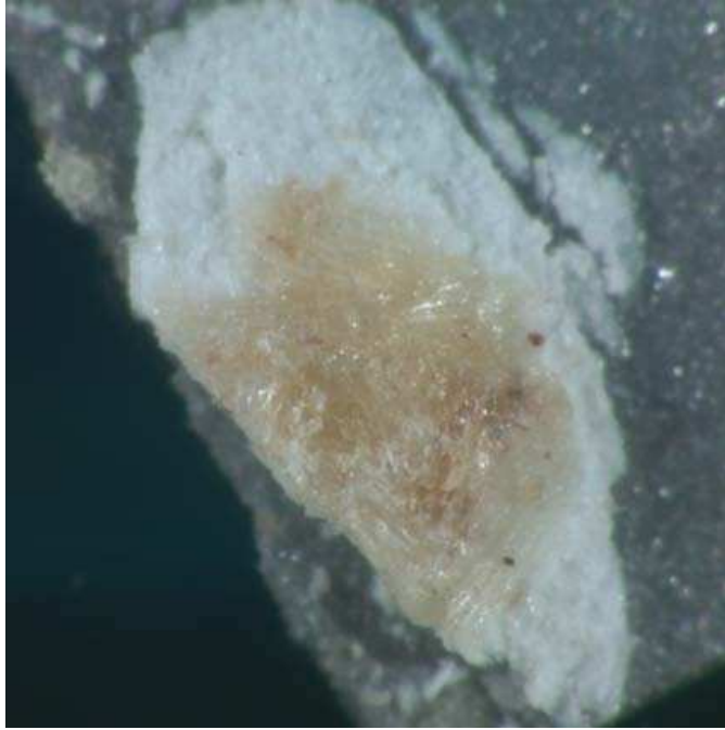
Figure 5. Light microscopy image x32 showing the particle removed during chipout.
