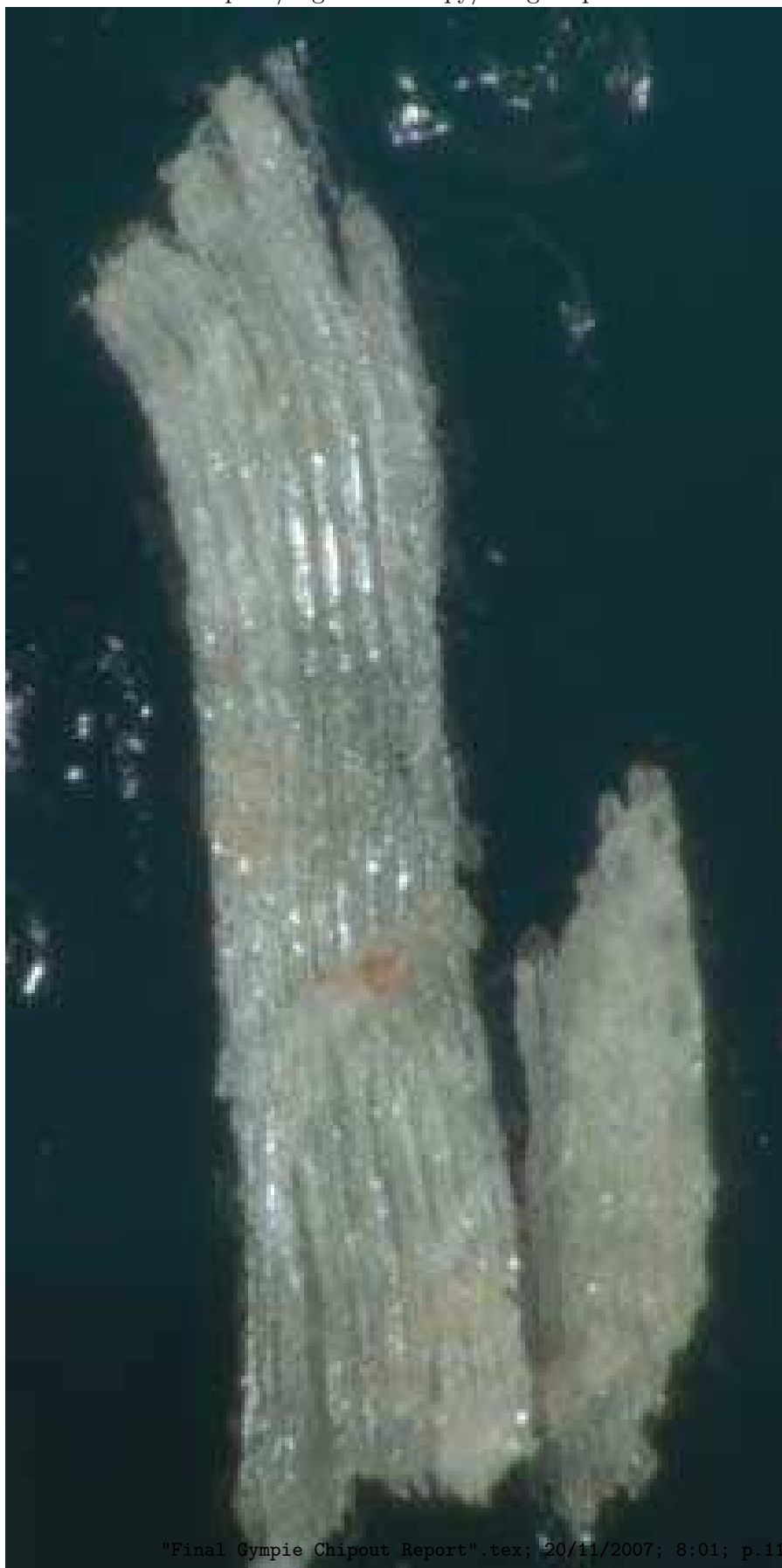
Figure 8. Light microscopy image x32 showing particle geometry of Gympie surface flake.
