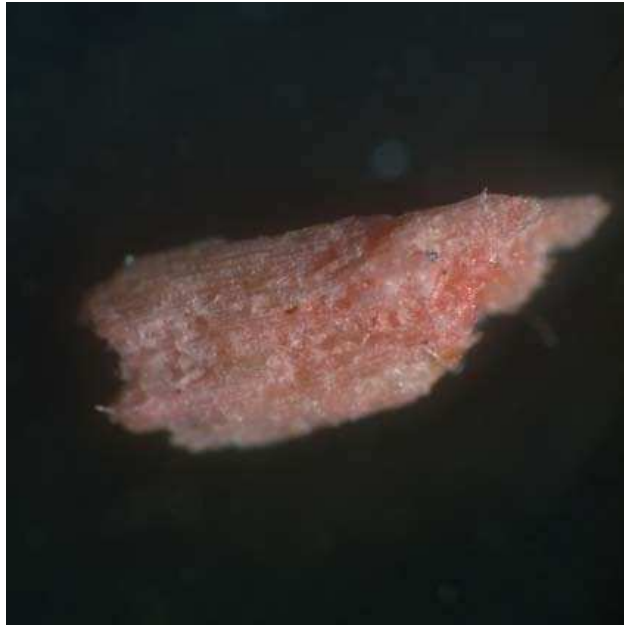
Figure 15. Light microscopy image x20 of blended surface flake ex the G1 spreaders showing little resination as seen by presence of red dye indicating little resin.
