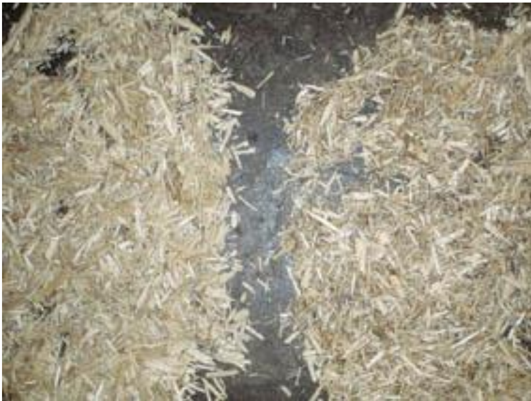
Figure 5 showing the effect of flake blended without Rezex A™ and with standard recommended blender settings, raw flake on the left of the image.
