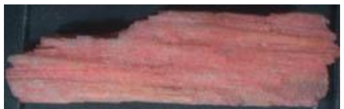
Figure 2: Image of poorly resinated flake in latter note resin coverage only around the edge
