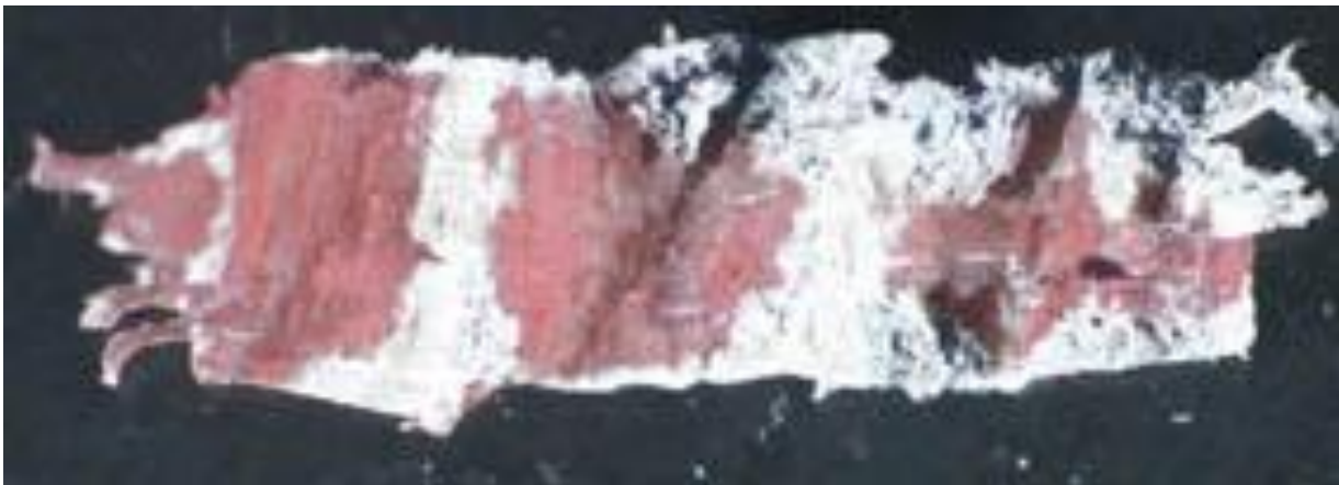
Figure 9 Image of stained core flake from Figure 8 through the first Stage of the binarisation process
