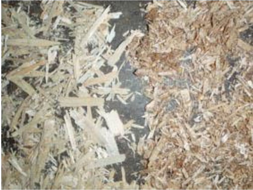
Figure 6 showing the effect of flake blended with Rezex A™ with modified blender settings, raw flake on the left of the image.
