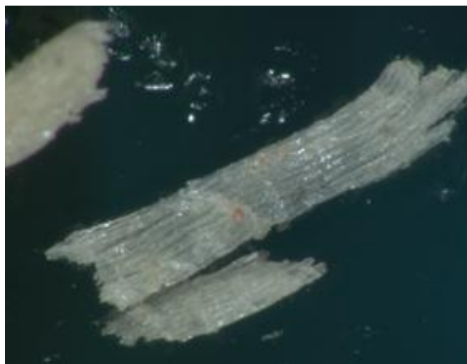
Figure 9 (x32) showing the high surface to volume (aspect) ratio
