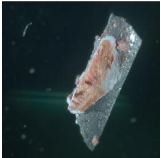
Figure 13 (x10) particle removed by chipout
