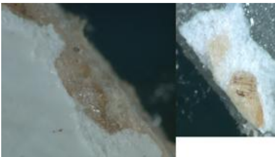
Figure 7 showing a chipout particle with sapstain fungus and associated void without
