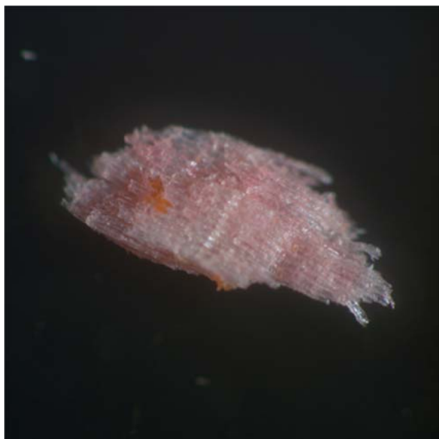
Figure 14 (x20) poorly blended surface flake as can be seen by the amount of Safronin O dye present
