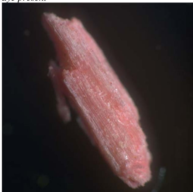
Figure 16 (x20) poorly blended surface flake
