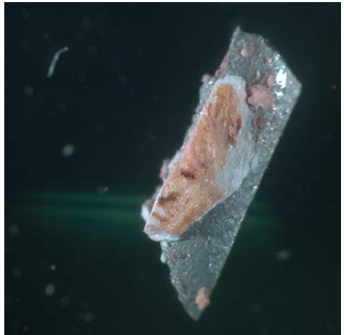
Figure 32 (x10) particle removed by chipout
