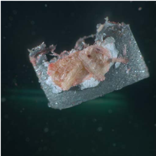
Figure 12 (x10) particle removed by chipout Note the presence of the Safronin O dye showing no resin distributed on the flake.
