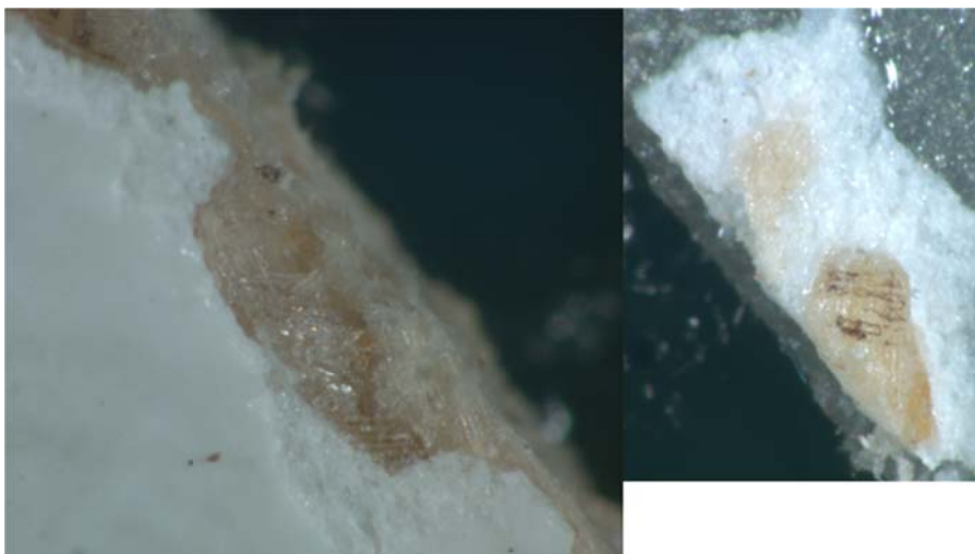
Figure 5 chipout particle and associated void
