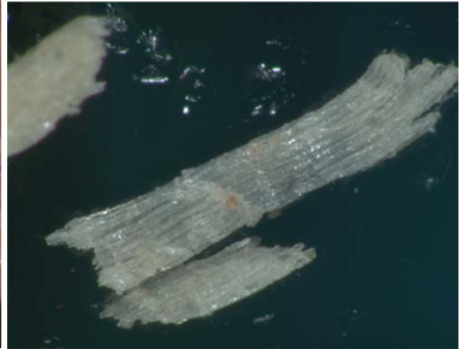
Figure 9 (x32) showing the high surface to volume (aspect) ratio
