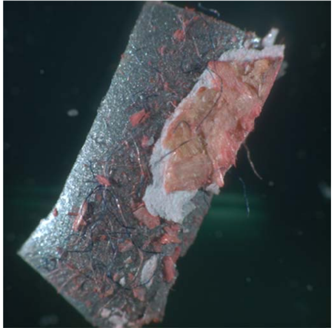
Figure 11 (x10) particle removed by chipout
