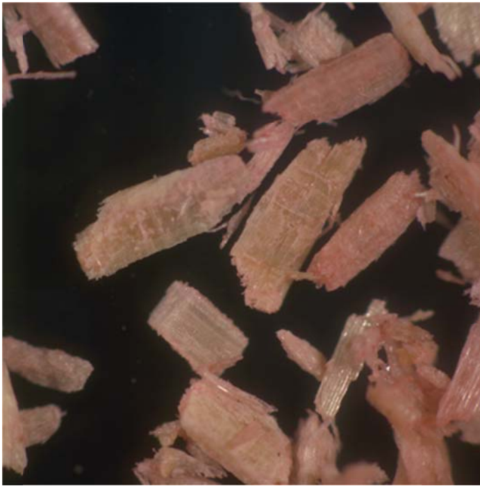
Figure 8 (x10) showing good particle geometry of the plant's surface flake
