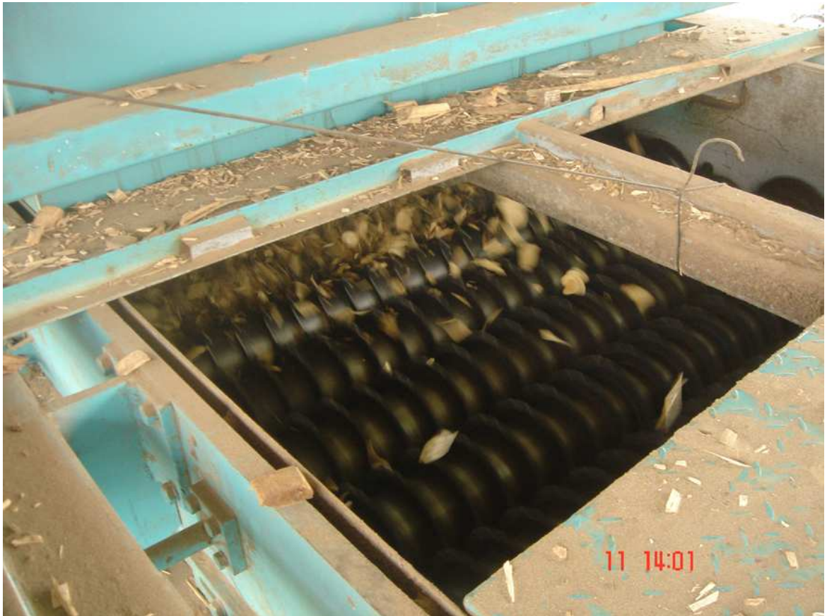
Figure 7. Discscreen removing oversized chips
