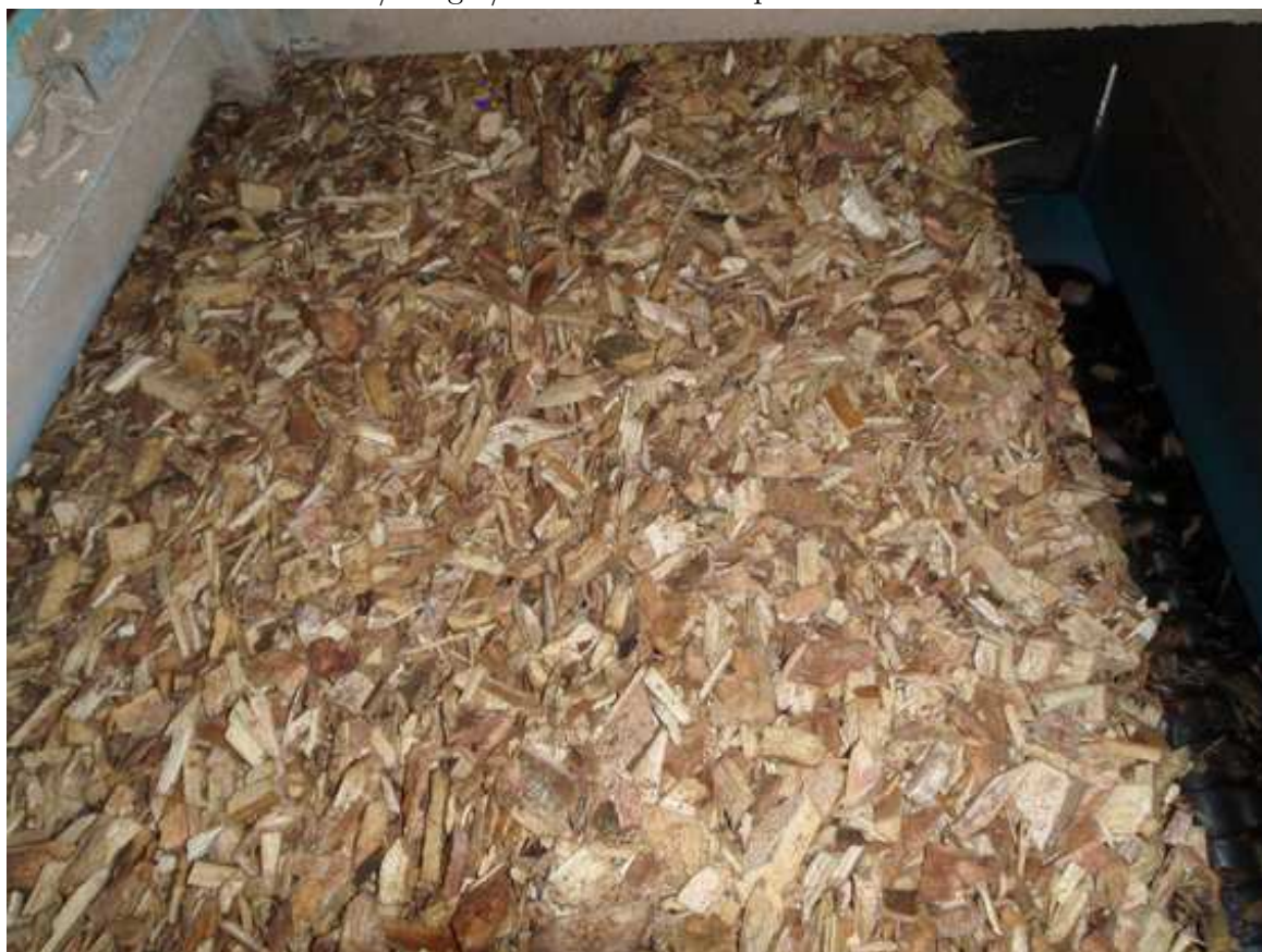
Figure 8. First stage of discscreen removing fines, note screen is grossly overloaded
