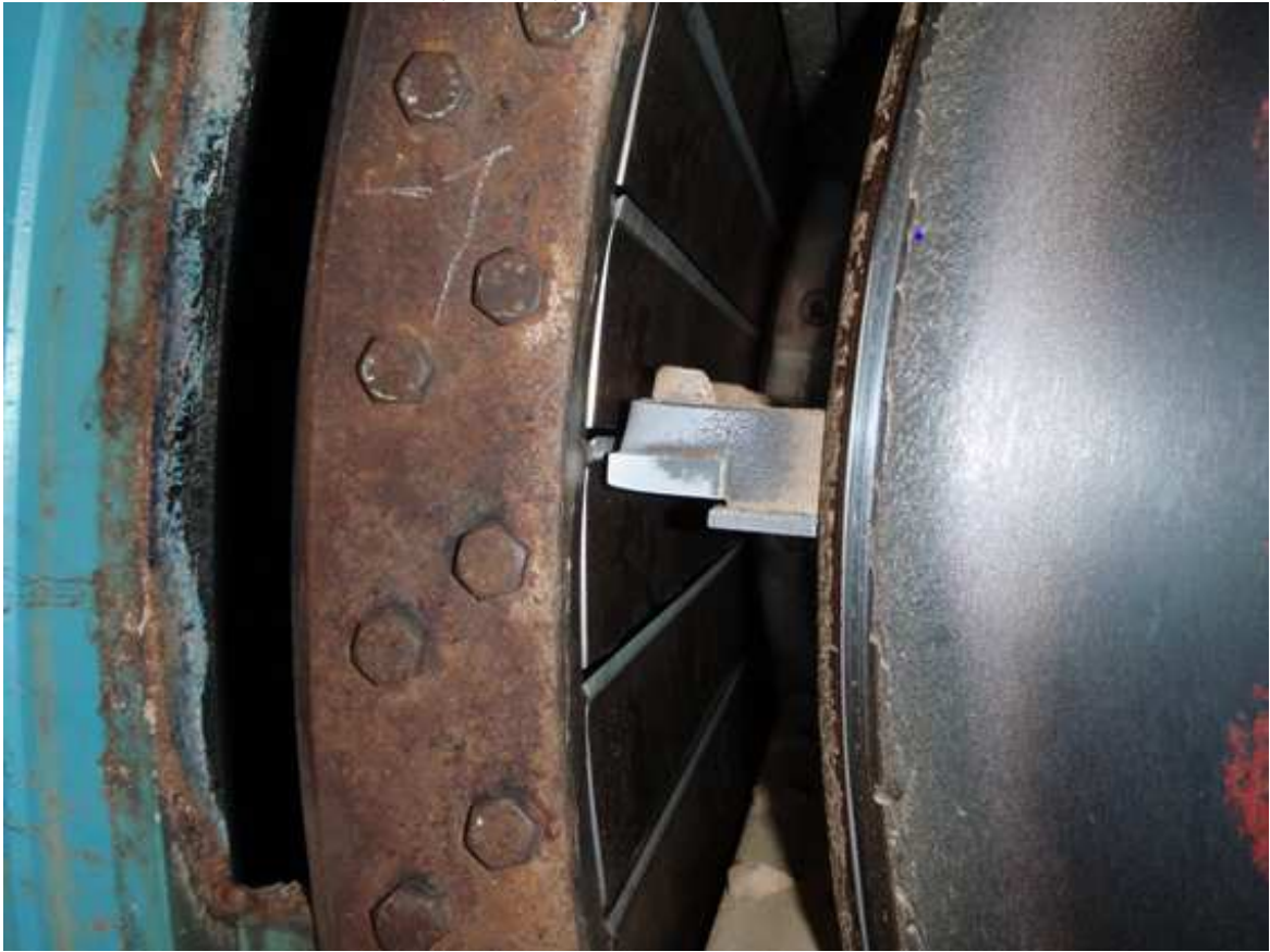
Figure 9. Close up image of flaker beaters showing wear at the corner and wear plates showing excessive wear
