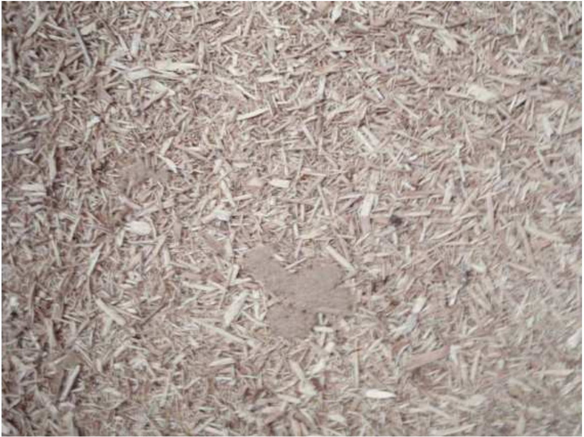
Figure 19. Dust spots in the mat prior to pressing.
