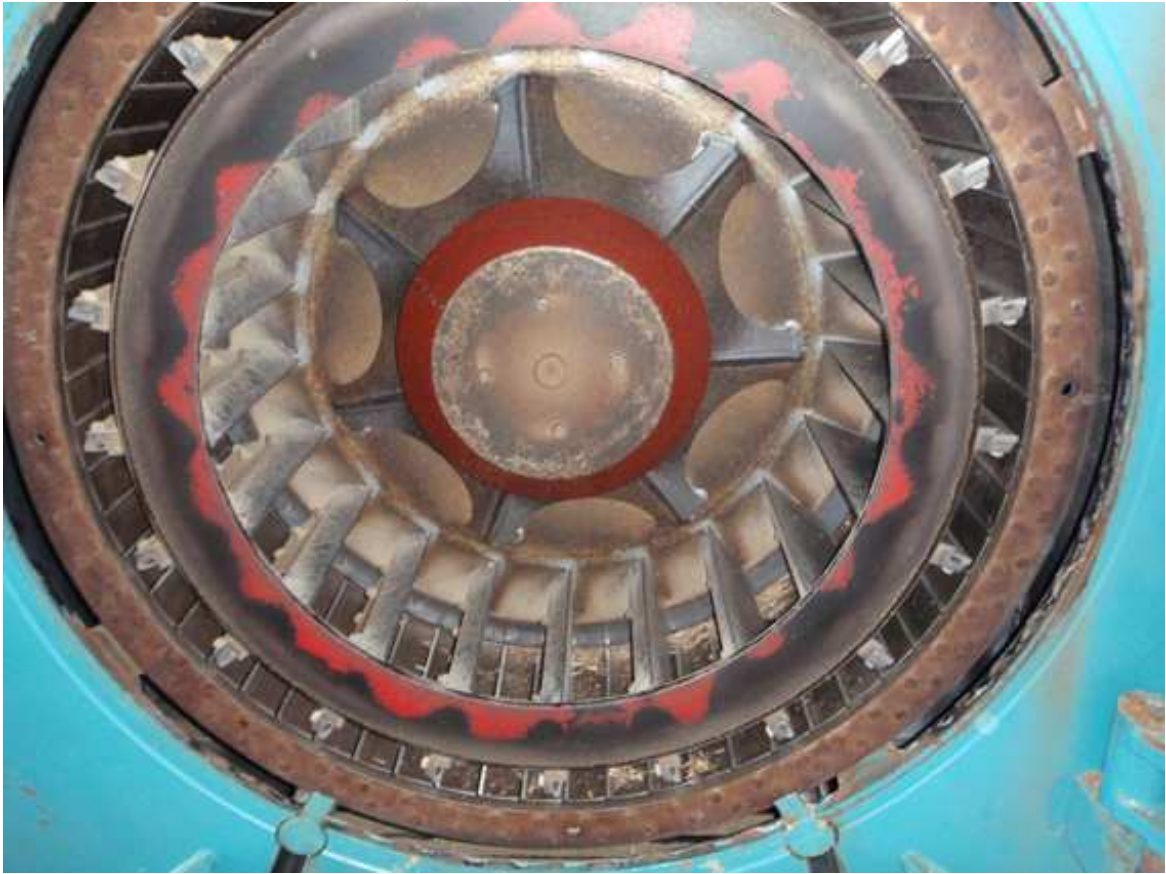
Figure 11. General configuration of the static knife ring in relation to the beaters
