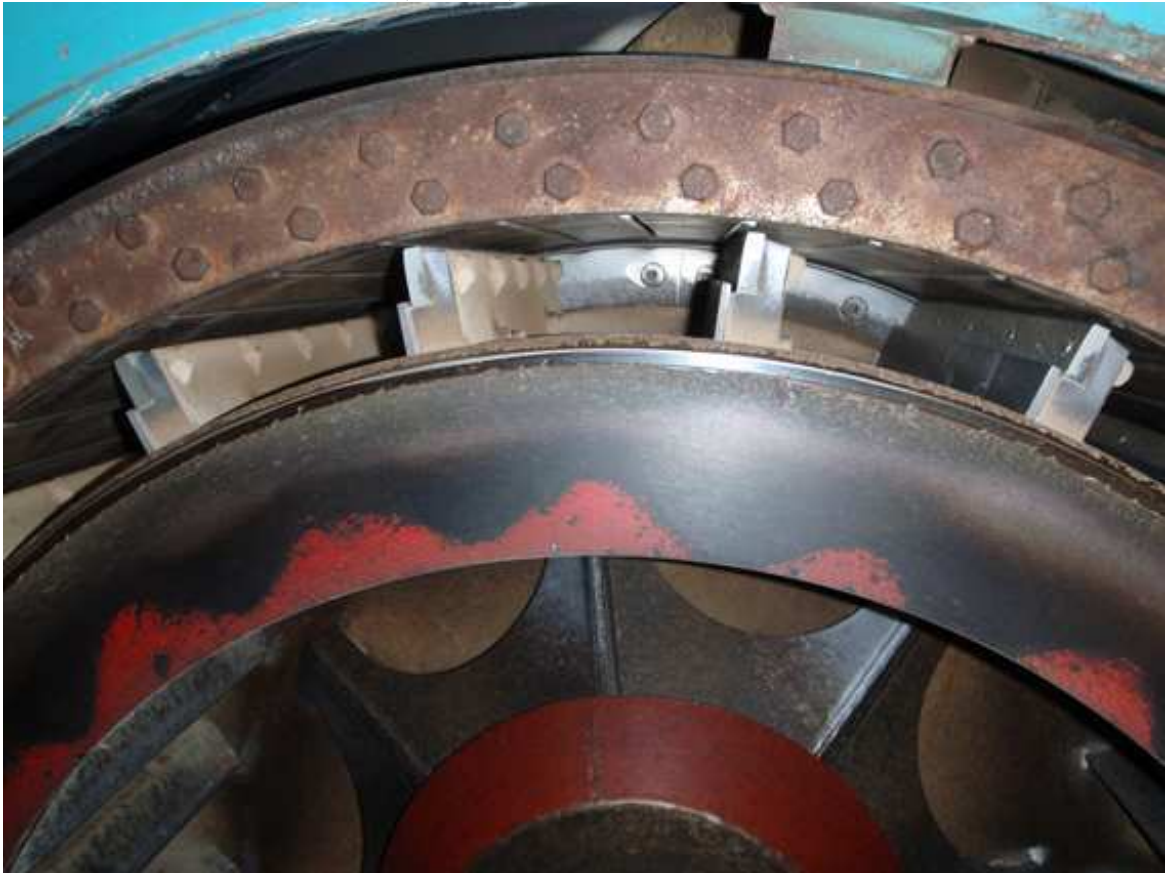
Figure 10. Image showing relative position of the beaters, knives and wear plates
