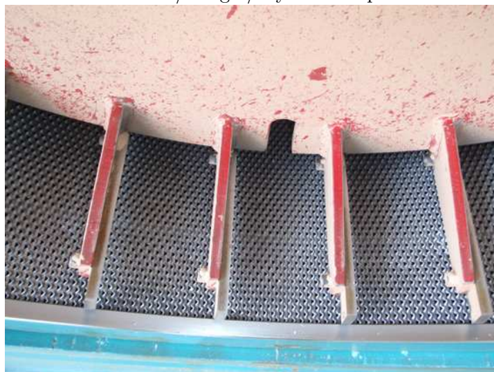
Figure 15. Images of the dry refiner showing screens and beaters
