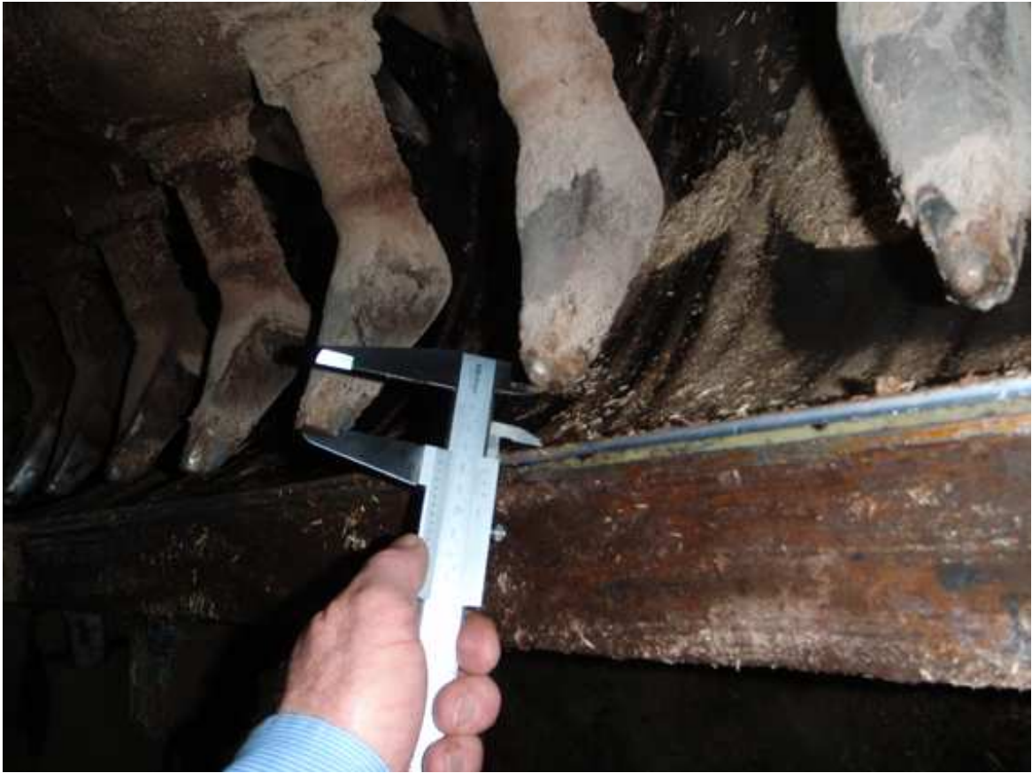
Figure 16. Note excessive distance between blender horn and shell of blender
