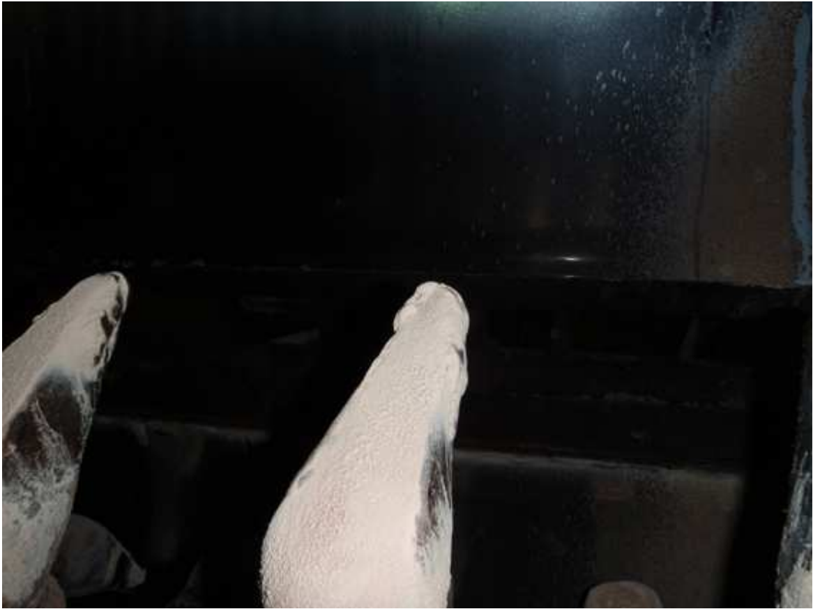
Figure 17. Image showing buildup of resin on blender horns due to insufficient cooling.
