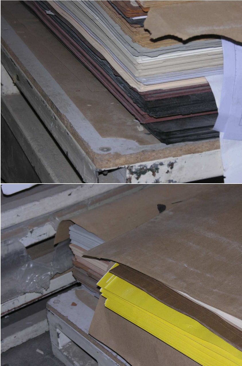
Figure 18. Images showing very poor stacking that will result in paper chips during lay-up
