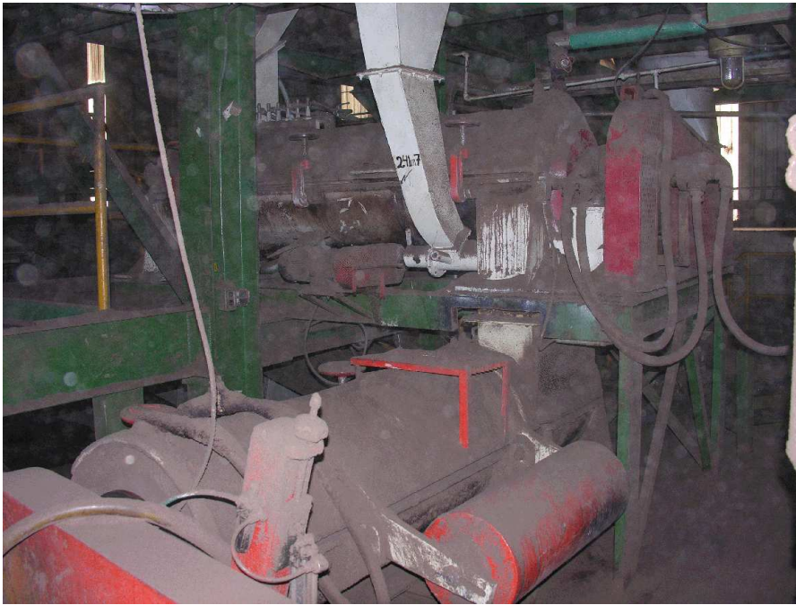
Figure 15. Configuration of the dust blender after the standard surface blender, note no injection nozzles.
