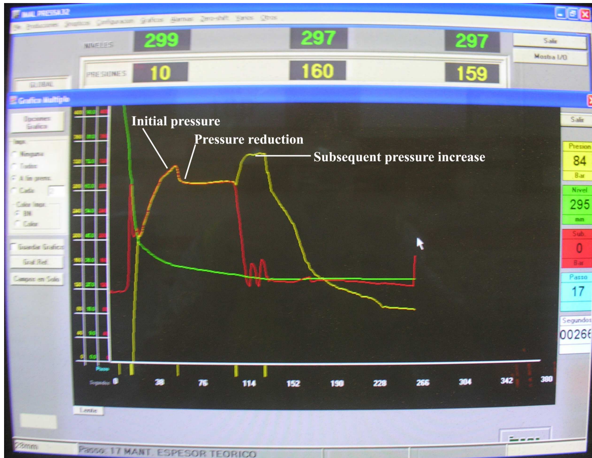
Figure 16. Press cycle showing pressure reduction after maximum pressure reached followed by a subsequent increase in pressure
