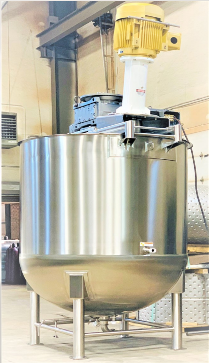
Twin Motion Kettle with Admix High Shear Mixer
