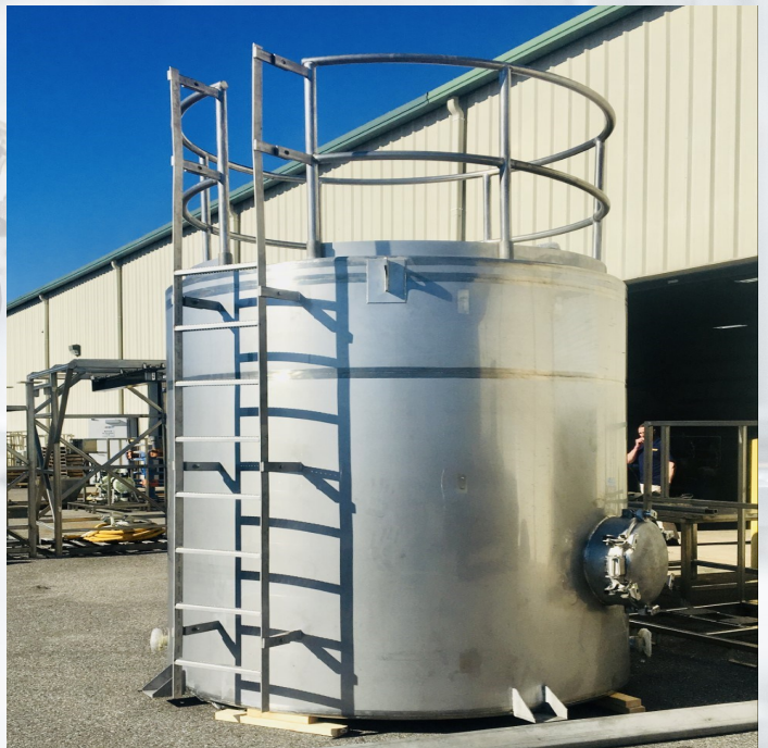
6,000 Gallons Capacity Storage Tank
