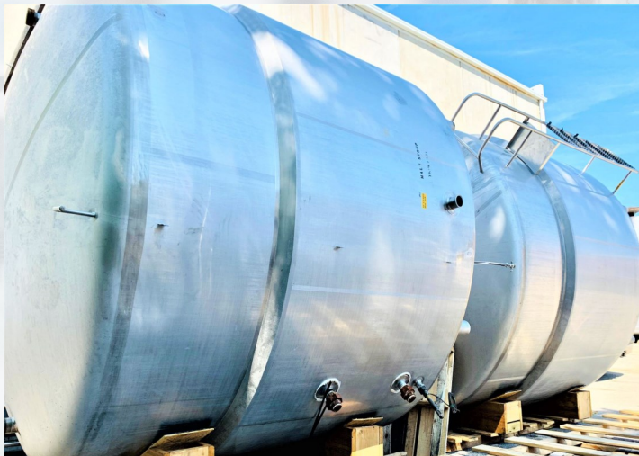
7,500 Gallons Storage Tanks
