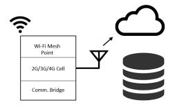
SimplBox is equipped with fault-tolerant networking and SimplWeb which is a real-time database hosted by Simpl Global.
