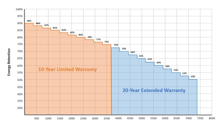
Aggregate Discharge Throughput (kWh throughput / kWh nameplate)
