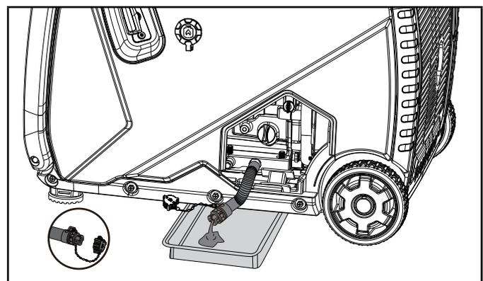
5. Replace the oil drain plug.
