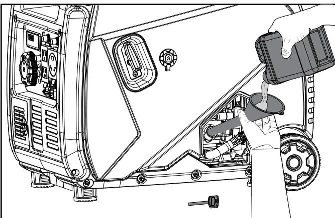
5. Check engine oil level before each use and add as needed.
