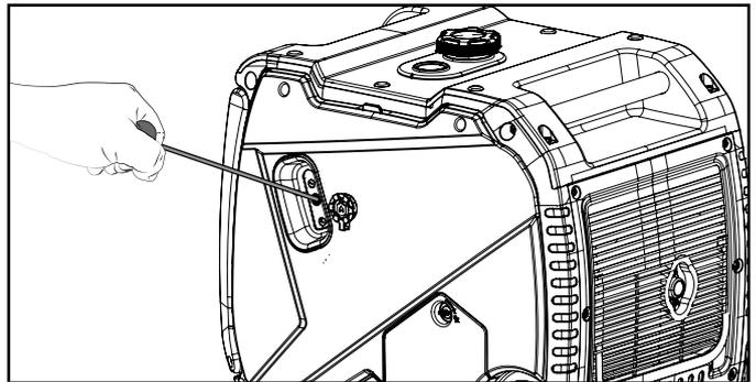
5. Do not over-choke. As soon as engine starts, turn the EZ Start dial to the "RUN" position.
