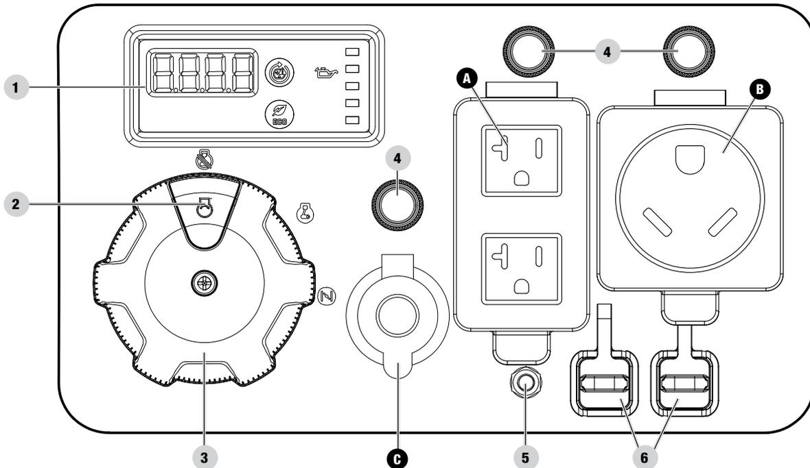
1. **Intelligauge with Power Meter** – See *Intelligauge with Power Meter* section.
