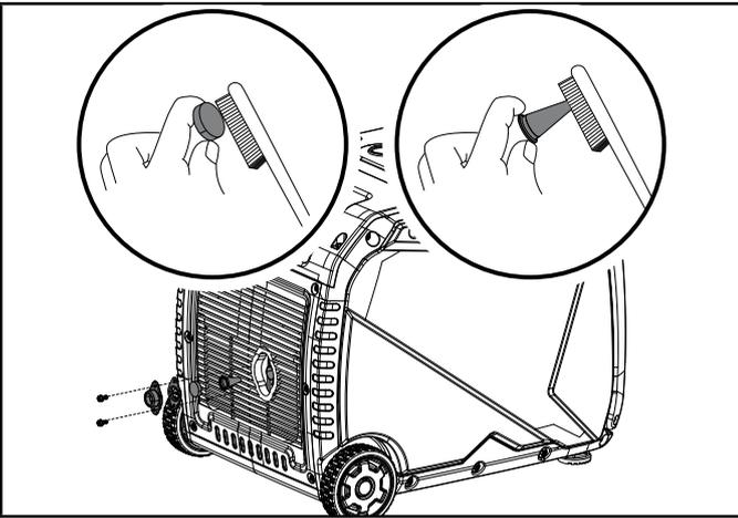
5. Replace the spark arrestor and spark arrestor screen if they are damaged.
