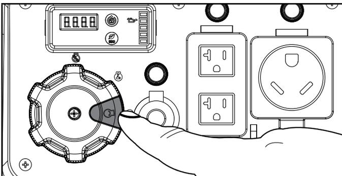
6. Do not over-choke. As soon as engine starts, turn the EZ Start dial to the "RUN" position.
