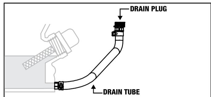
4. Ensure the oil drain hose is lower than the engine and allow the oil to drain completely into an appropriate container.
