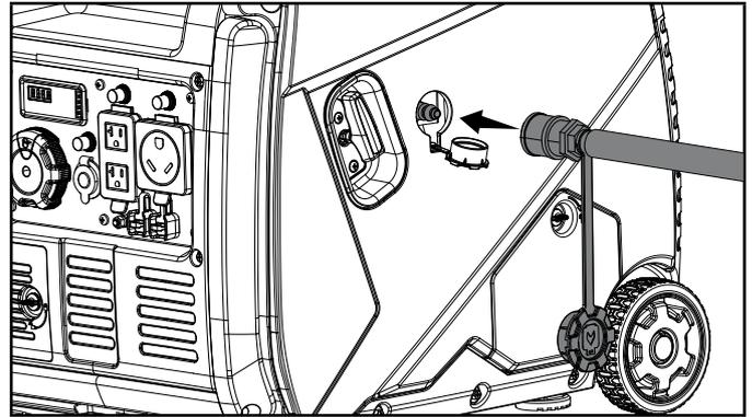
7. Check all connections for leaks by wetting the fittings with a solution of soap and water. Bubbles which appear or bubbles which grow indicate that a leak exists. If a leak exists at a fitting then turn off the valve on the cylinder and tighten the fitting. Turn the valve back on and recheck the fitting with the soap and water solution. If the leak continues or if the leak is not at a fitting then do not use the generator and contact customer service.
