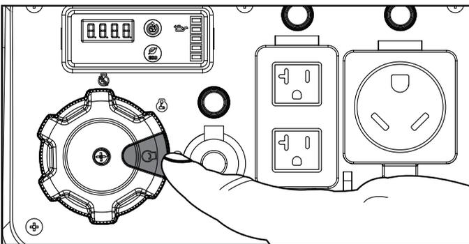
5. Do not over-choke. As soon as engine starts, turn the EZ Start dial to the “RUN” position.
