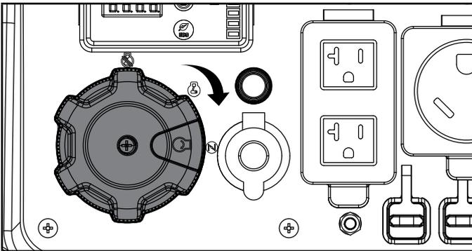
4. Press and hold the yellow ignition switch on the EZ Start Dial toward the center of the dial. Release as the engine begins to start. If the engine fails to start within five seconds, release the switch and wait at least ten seconds before attempting to start the engine again.
