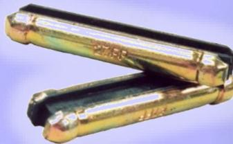
The H&L® Flexpin® consists of two half-round lengths of steel with a section of live rubber vulcanized between to form an oval shaped pin. The compressed rubber forces the Flexpin® half-round section in opposite directions. See webpage for all Flexpin updates and dimensions T163.2016.
