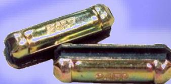
The H&L® Flexpin® consists of two half-round lengths of steel with a section of live rubber vulcanized between to form an oval shaped pin. The compressed rubber forces the Flexpin® half-round section in opposite directions. See webpage for all Flexpin® updates and dimensions T163.2016.
