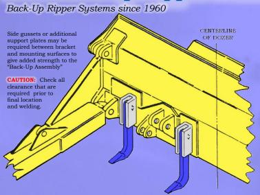
As the tractor moves forward, the ripper assembly drag freely behind the dozer blade and as the tractor moves to the rear each shank falls into the ripping position. Rippers become inoperative by simply raising the shank assembly up and inserting the pin in the "Back-Up Ripper" bracket.
