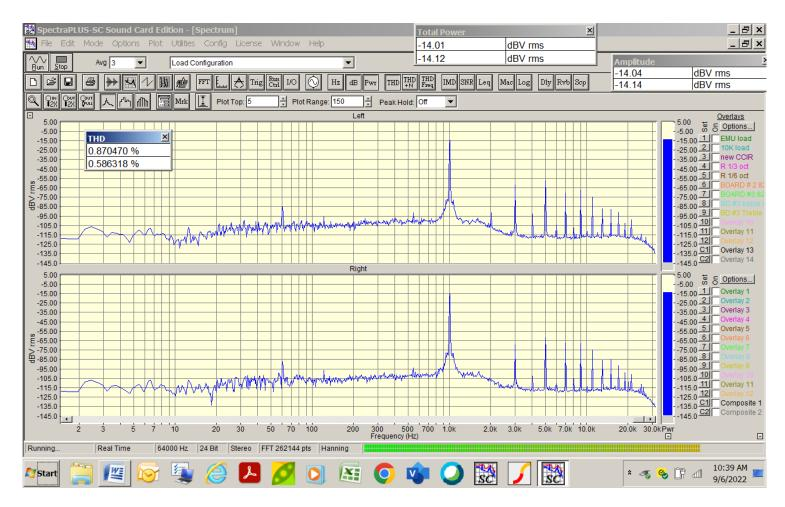
+13 dB re 350nW/m (+14 dB re 320nWb/m) indicates less than 1/3 to 1/5 the Total Harmonic Distortion specified by the Tape Manufacturer (3% 3rd Harmonic Distortion) at this level. (-21 dB Single-Ended measurement PAD on Repro Card output).
