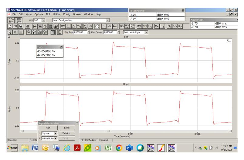
1 Khz wideband (192Ks/s Digitally-generated IIR-filtered) Square Wave 15ips CCIR, approx -3 dB below 350nW/m.
