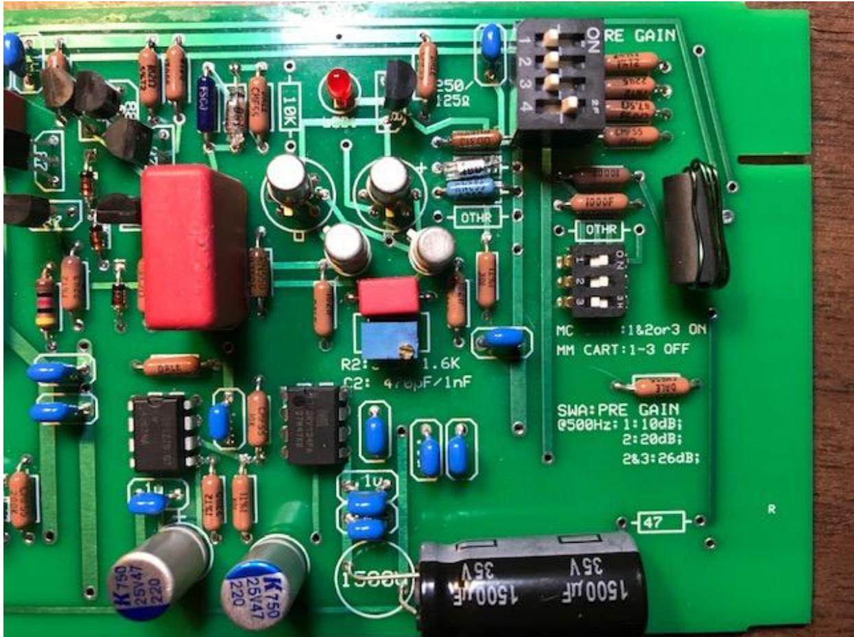
**1. Cartridge Type (MM or MC) and LOADING:**
