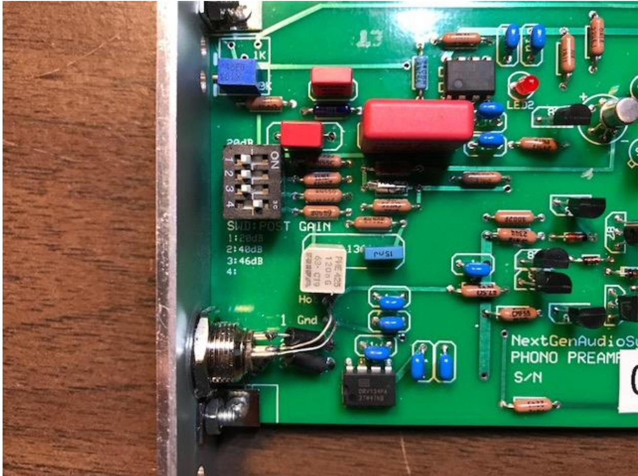
**Output Stage Gain settings: ONLY ONE SWITCH SHALL BE SELECTED ON AS FOLLOWS**
