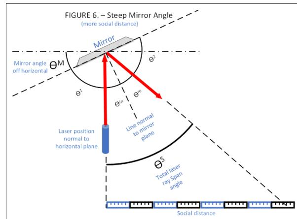
the system by moving the mirror from a shallow angle to a steep angle off the horizontal plane.
