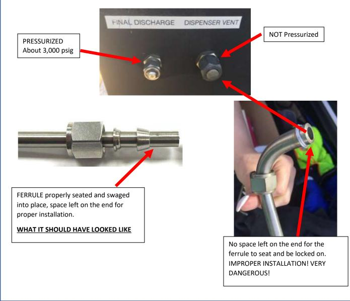
What Happened (cont'd): The technician had just touched his wrench to the high-pressure fitting in an attempt to turn the nut and bleed down the small section of pressurized tubing so that he could completely remove the nut and check the ferrule and installation. As soon as he touched it, it came apart in a violent manner ejecting gas and immediately bending the tubing. It made a loud "Pop" sound followed by the distinct sound of gas pressure being relieved.
