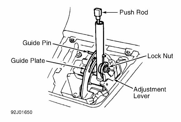
Fig. 4: Identifying Gearshift Lever Components Courtesy of MAZDA MOTORS CORP.
