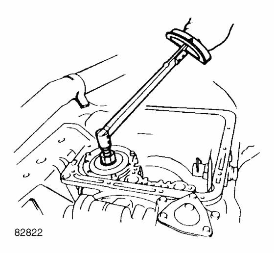
Fig. 1: Adjusting 2nd Gear Brake Band Courtesy of MAZDA MOTORS CORP.
