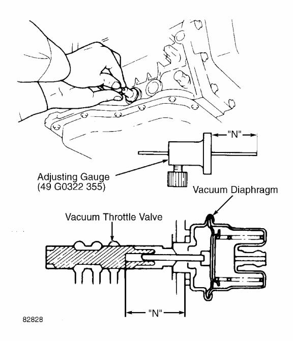
Fig. 6: Checking Vacuum Diaphragm Rod Length Courtesy of MAZDA MOTORS CORP.
