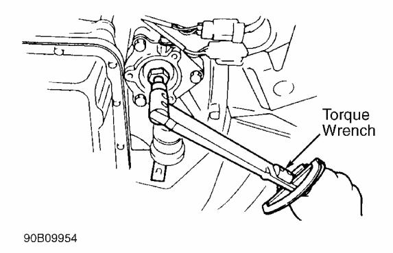
Fig. 2: Adjusting Overdrive Band Courtesy of MAZDA MOTORS CORP.
