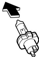
10. Install the new socket and bulb assembly in the reverse order of removal.
