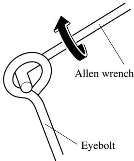
4. Disconnect the eyebolt from the Allen wrench leaving the Allen wrench in place, and insert the threaded end of the eyebolt in the hole directly above the Allen socket and tighten it clockwise two full turns.
