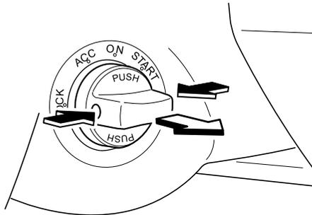
4. Insert the auxiliary key in the ignition switch.
