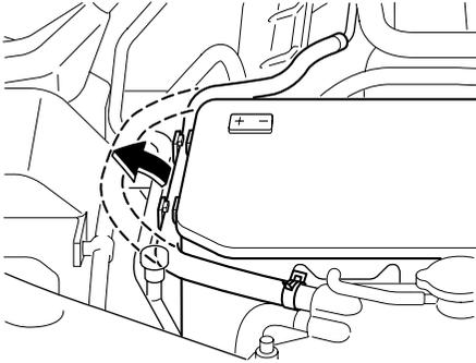
2. Remove the battery cover from its right side.
