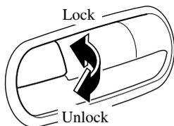
To lock any door with the door-lock knob from the outside, push the door-lock knob to the lock position and close the door.
