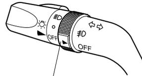
To turn them off, rotate the fog light switch to the OFF position or turn the headlight switch to the
