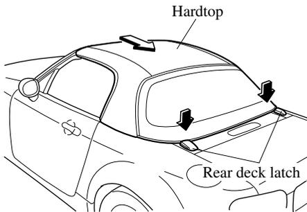
13. Lift the hardtop straight off the body to prevent damage to the rear deck latches and studs.
