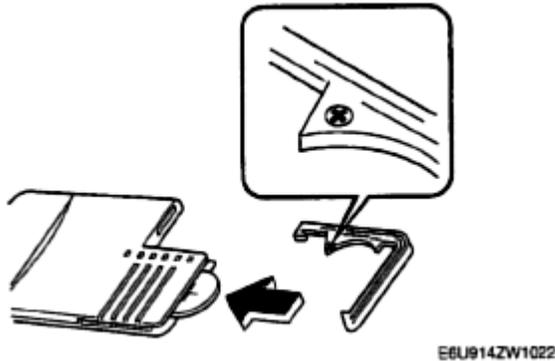
**Fig. 37: Positions For Inserting New Battery**
