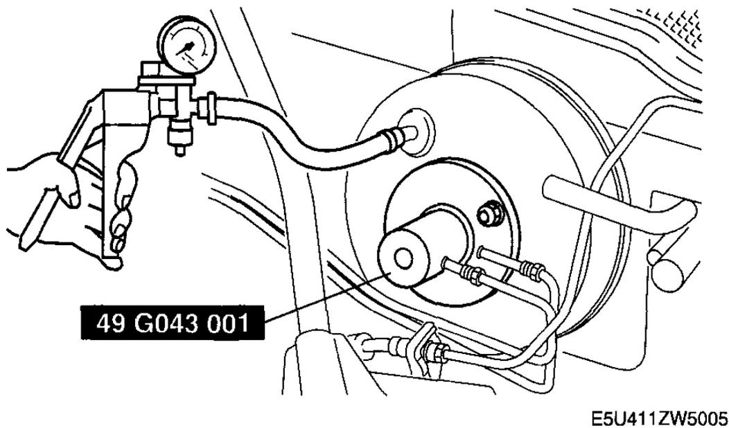
**Fig. 13: Applying Vacuum To Power Brake Unit Using Vacuum Gauge**
