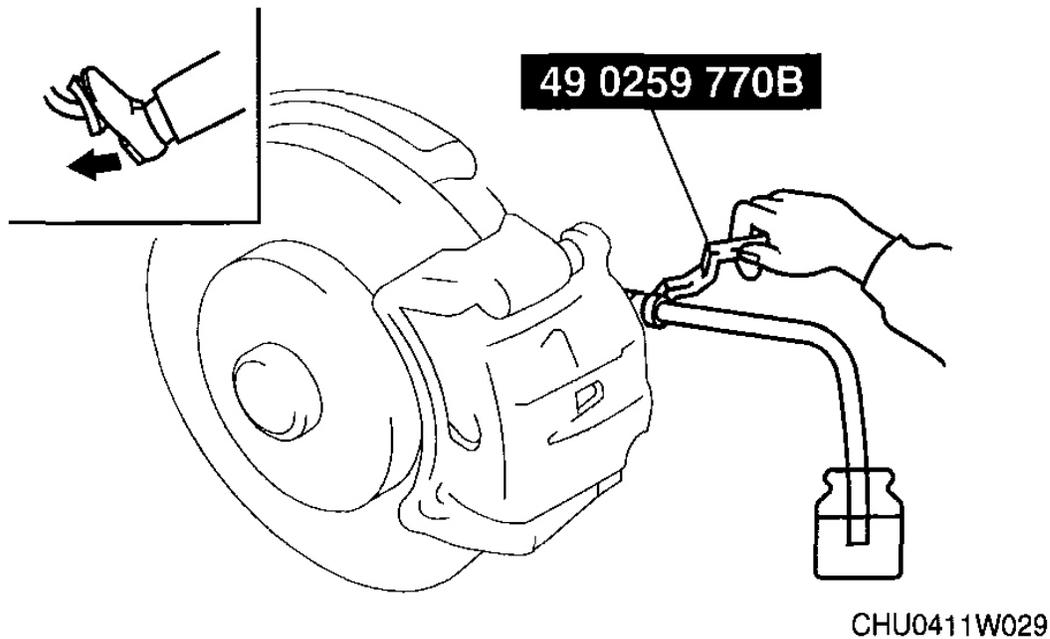
**Fig. 2: Brake Bleeding Procedure**
