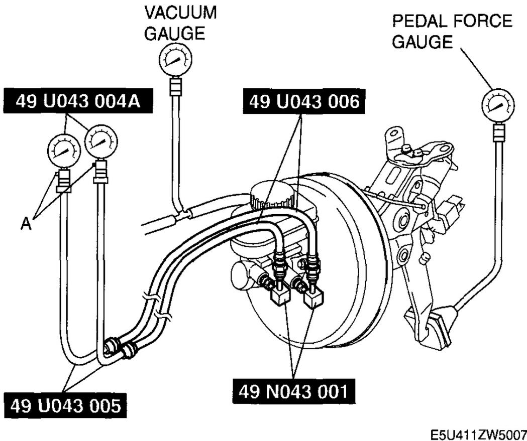
**Fig. 20: Inspecting Vacuum Loss Function - With DSC**
