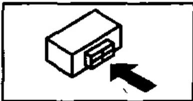
**Fig. 17: Identifying Brake Fluid Level Sensor Connector**
