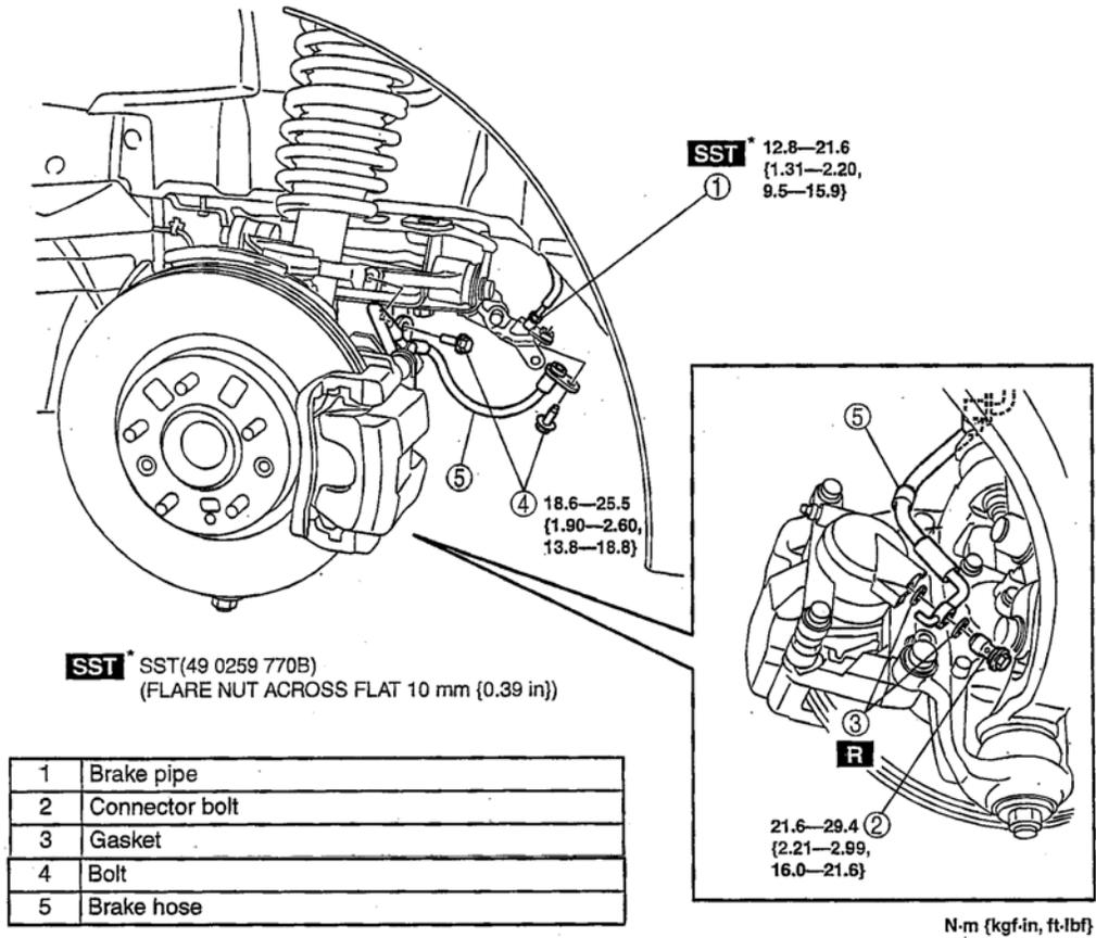
**Fig. 53: Identifying Brake Hose (Front) Components (With Torque Specifications)**
