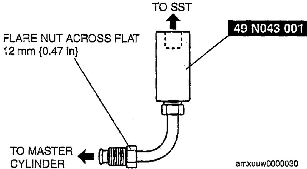
**Fig. 18: Installing SST (49 N043 001)**
