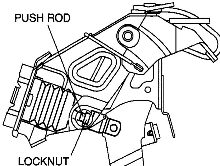
**Fig. 5: Adjusting Brake Pedal Height**
