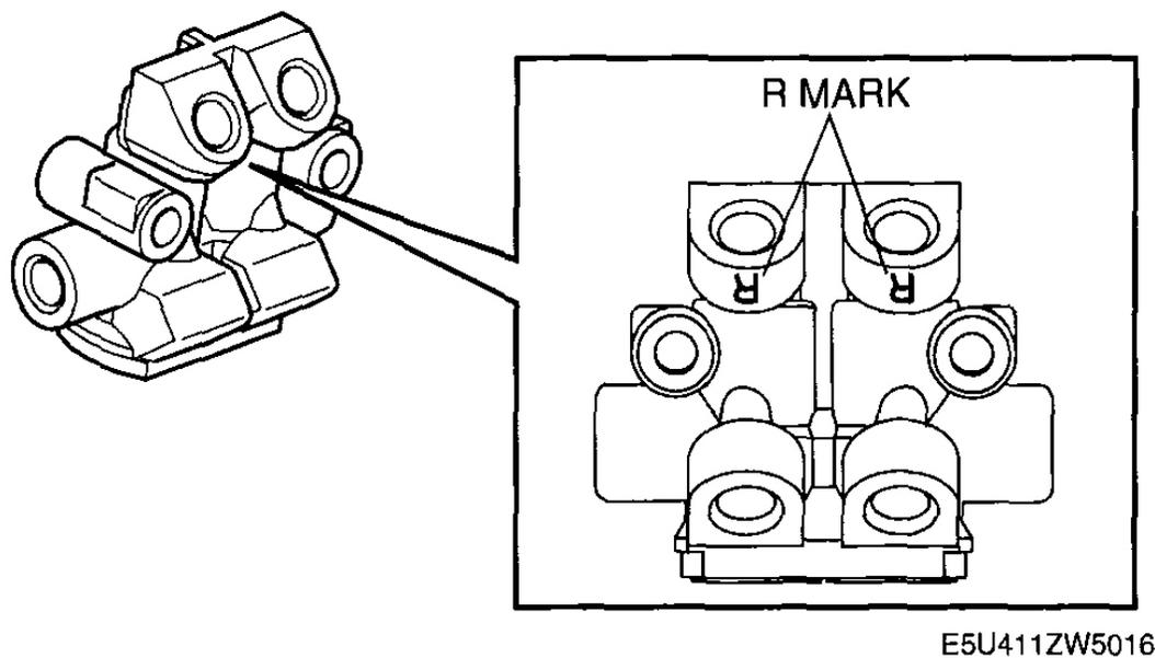
**Fig. 26: Identifying Dual Proportioning Valve R Marks**
