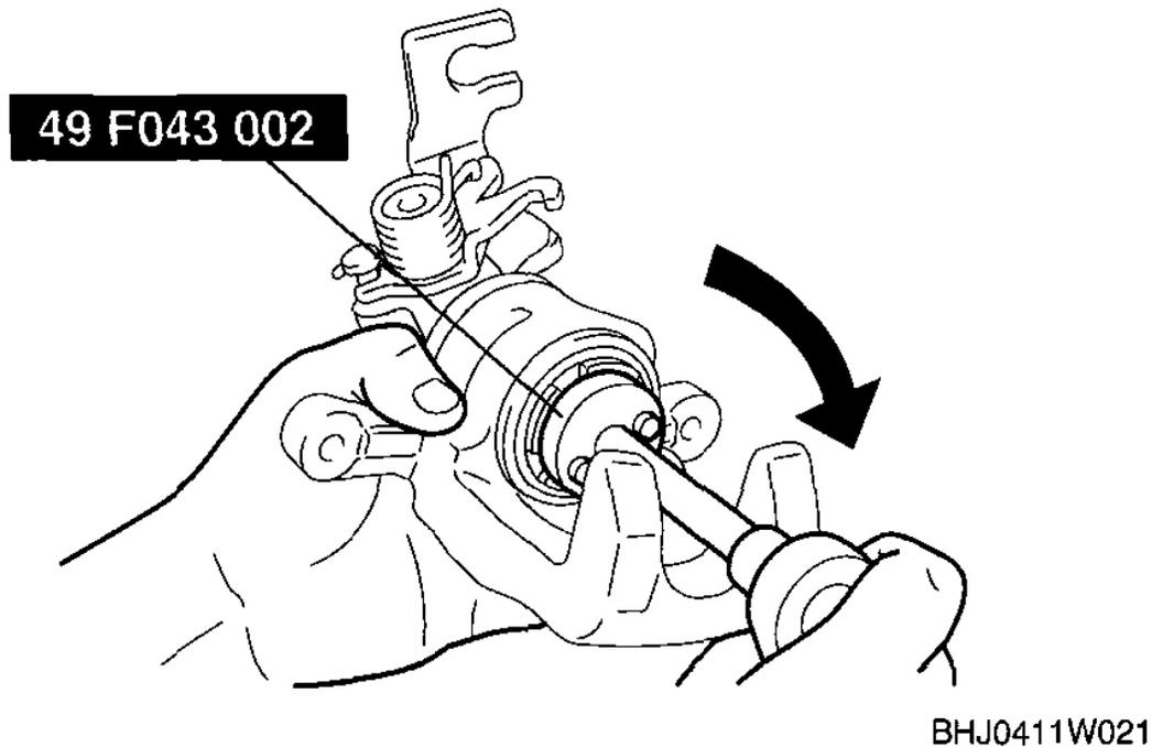
**Fig. 52: Rotating Piston Clockwise Using SST**
