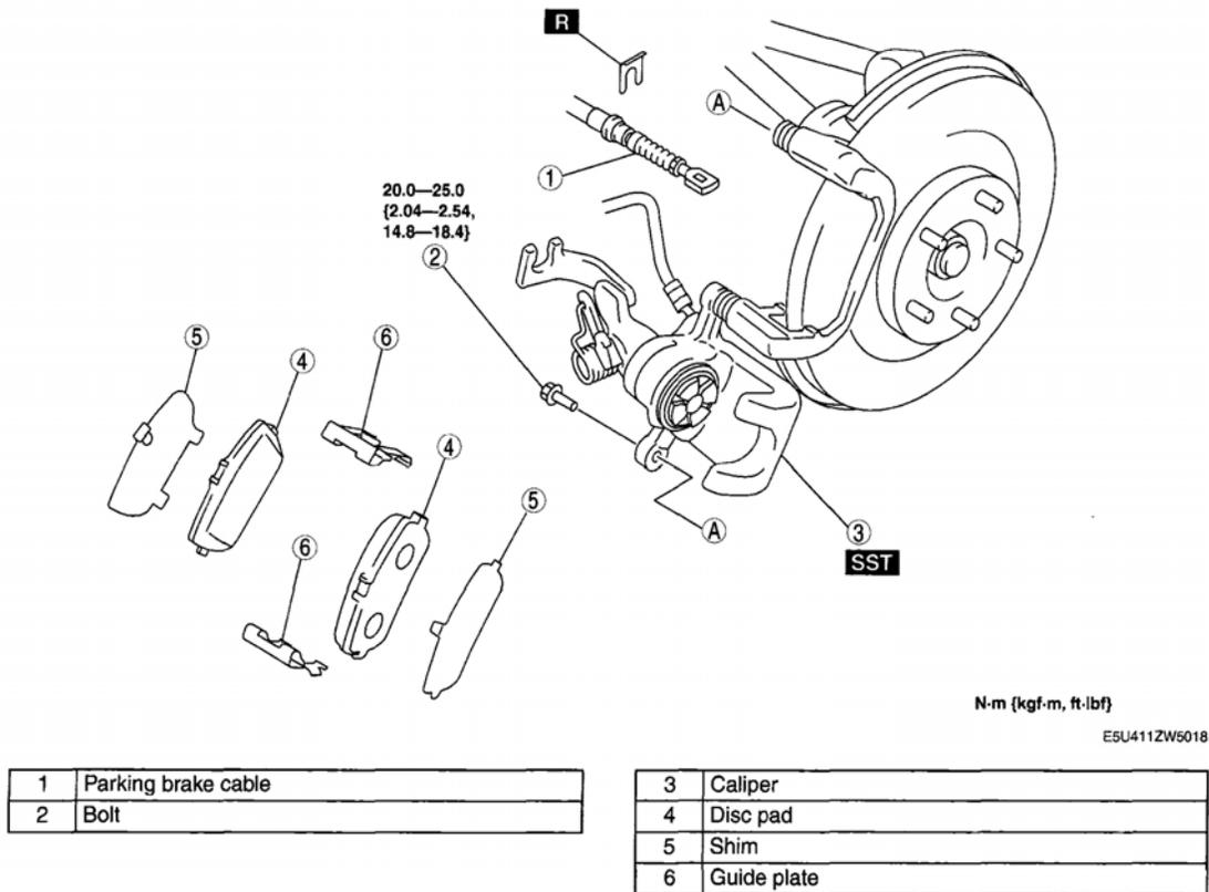
**Fig. 47: Identifying Disc Pad (Rear) Components (With Torque Specifications)**
