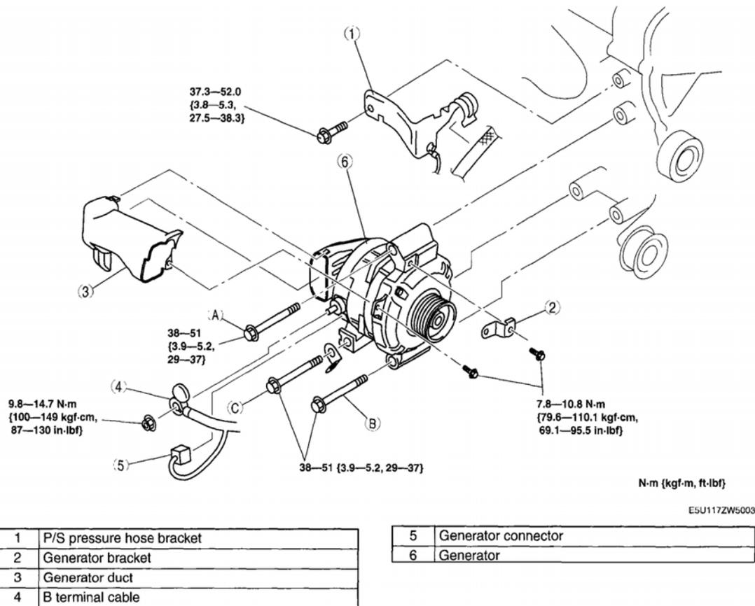
**Fig. 7: Identifying Removal Order Of Generator (With Torque Specifications)**
