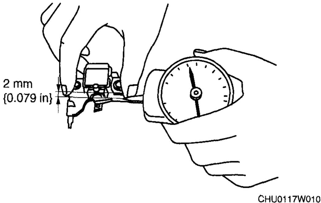
**Fig. 16: Measuring Force Of Brush Spring Using Spring Pressure Gauge**
