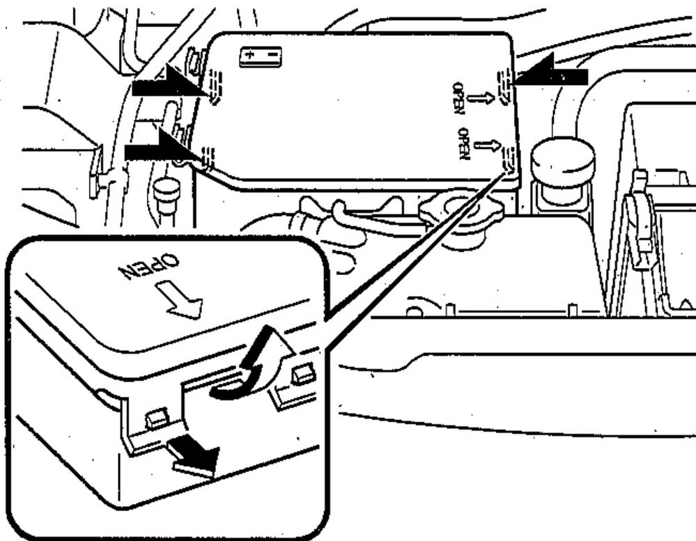
**Fig. 4: View Of Right Side Battery Cover**
