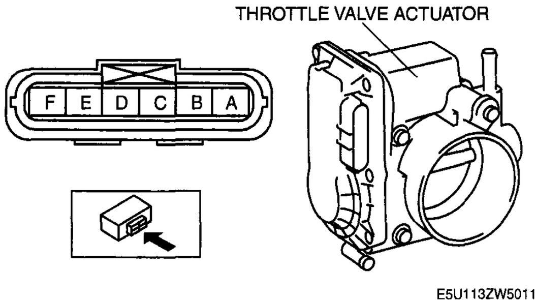
**Fig. 14: Identifying Throttle Actuator Connector Terminals**
