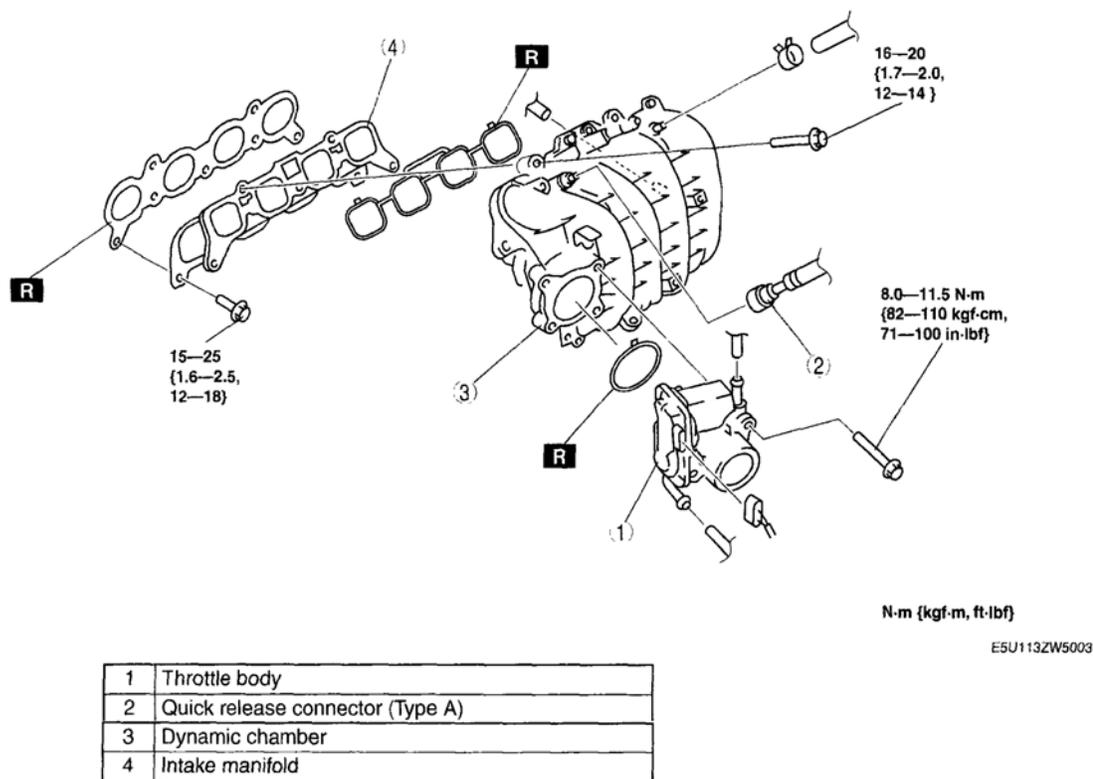
**Fig. 5: Identifying Removal Order Of Intake-Air System (Step 2) (With Torque Specifications)**
