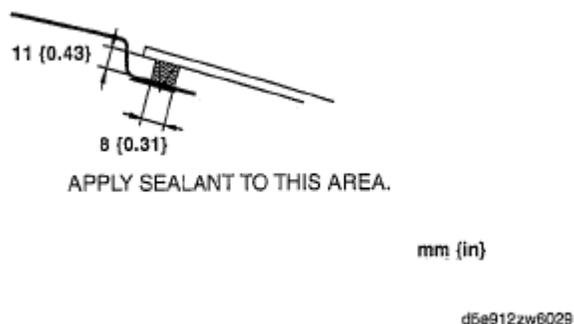
**Fig. 45: Identifying Sealant Applying Area On Glass Surface**
