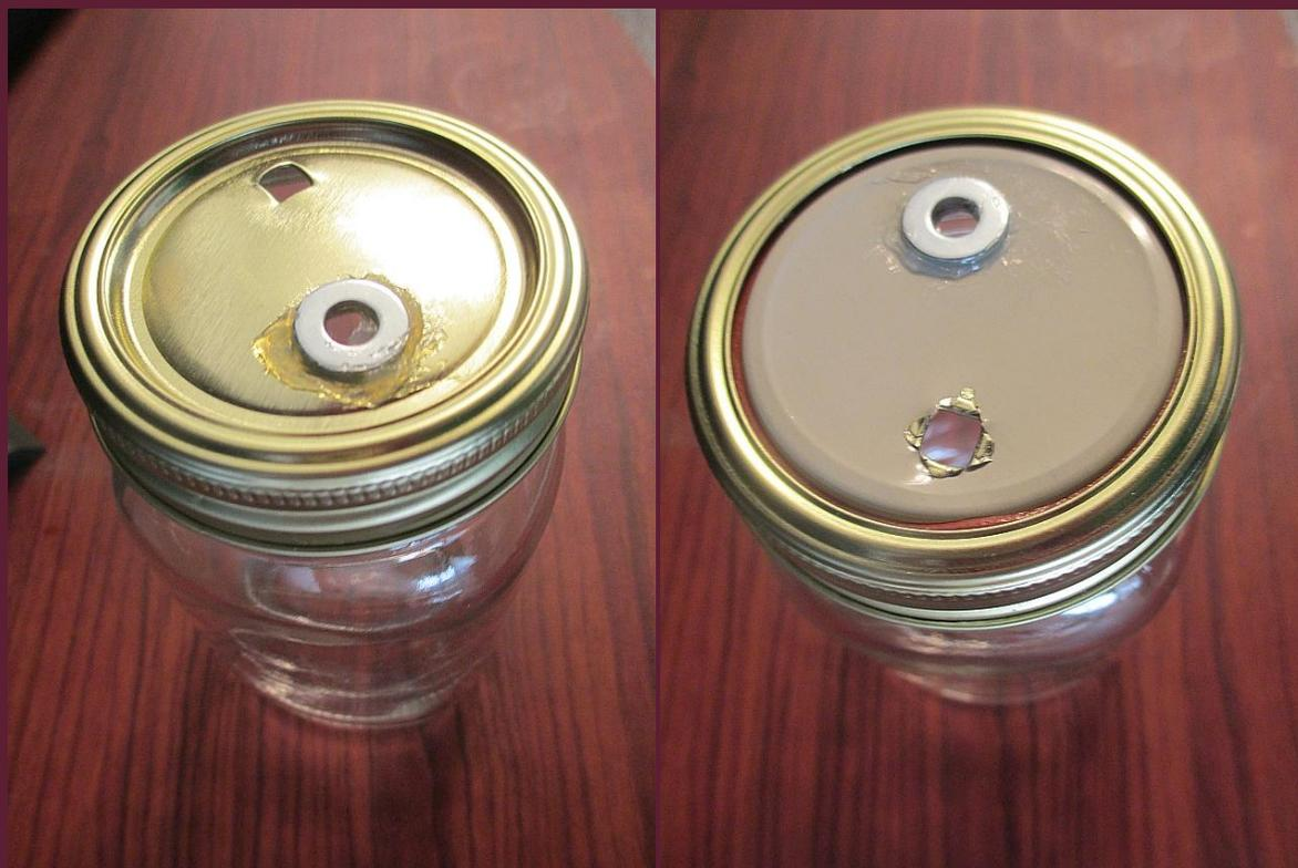
Put a little more silicone on each washer and then put a tyvek circle on each one, making sure that they are fully sealed to the washer and also that the hole in the lid remains open.
