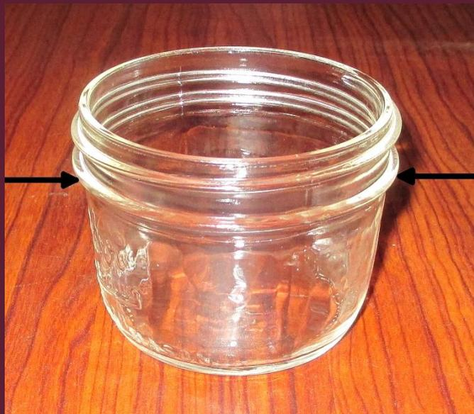
*Fill each jar with substrate no higher than the arrows in this picture*
