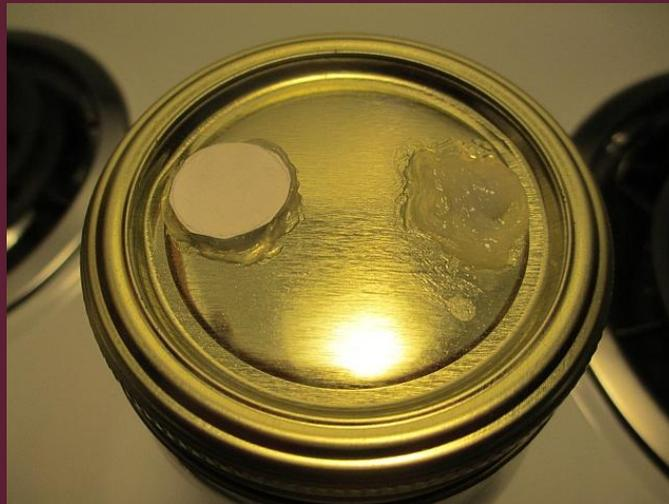
*A finished lid for use with spore water or liquid culture, with the tyvek filter on the left*
