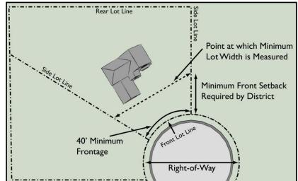
Cul-de-sacs shall meet the minimum design standards of the County Road Commission. A cul-de-sac shall be determined to commence at the intersection of the radius of the cul-de-sac with the street right-of-way line. See graphic.
