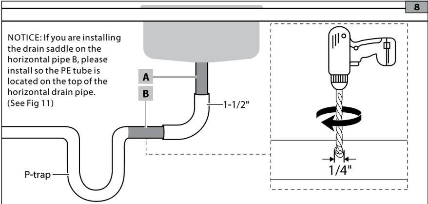
3. Drill a 1/4" hole. Make sure to only drill through one side of the drainpipe (Fig.8).
