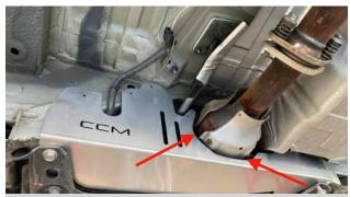
Do not fully install mid shield until the gap between the converter has been adjusted if necessary. A 7/16" Gap is adequate.
