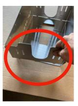
The tabs on each end should extend out from each end cap as shown here. There are 3 tabs on each side. The other 2 tabs on the bottom do not get bent.
