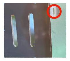
Once the tabs are though the slots, secure the pieces together by bending the tabs over as shown here. The tabs should look as pictured once they are installed properly. Set the lower box aside until top plate is installed.
