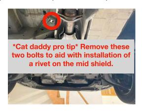
Due to variations with the exhaust, trimming of the mid shield may be required. Install mid shield without hardware and check for clearance around the converter. Mark contact areas, remove and trim shield. (We have found a grinder is quickest) Once the proper gap is obtained finish the installation.
