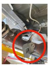
You will remove all of the factory bolts on the heat shield and discard. They will be replaced with (4) M6 Tamper-proof Torx bits, lock washers and flat washers, in that order.
