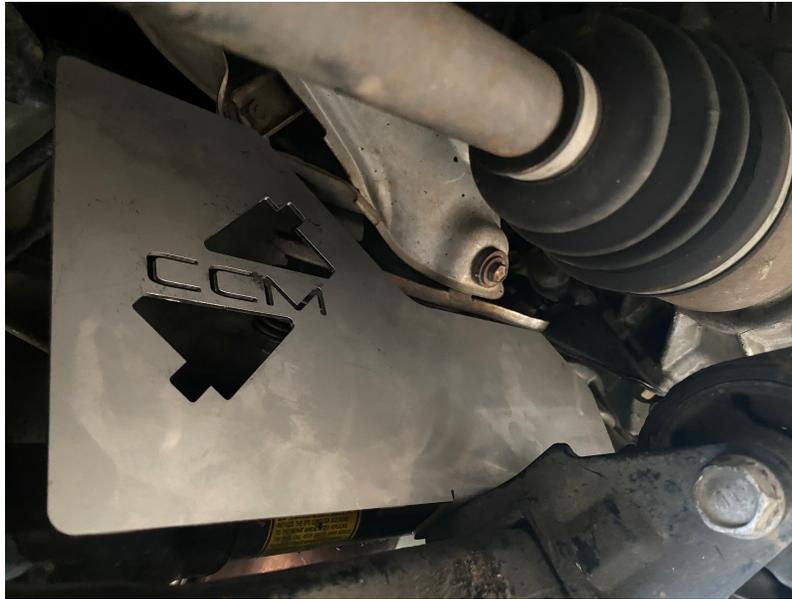
Step 2: Place the large rear shield and align the two outer corners on the subframe. (red mark on the black rivets) Secure the two front outer holes with these rivets.
