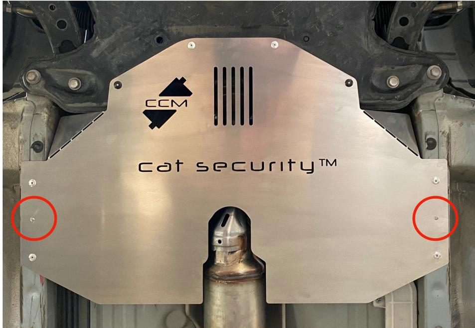
Step 4: Drill (6) 3/16" holes into the remaining holes. Then install the remaining rivets.
