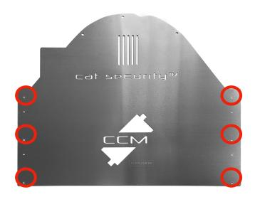
Step 5: Replace the front splash shield and tighten down the (3) 10mm nuts. Remove the clearance tool from between the cat and shield.
