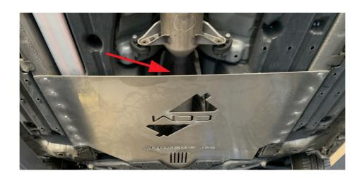
Step 3: Alternating sides, drill out the remaining holes. You can use the self tapping screws or a 3/16" drill bit. Once drilled, alternate sides again and install the rivets highlighted in the red areas.
