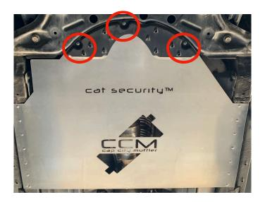
Step 2: The provided self-tapping screws to hold the plate in place while drilling the rivet holes. Place one security screw in any of the red outlined areas. These areas will house the security screws once the other holes for the rivets have been drilled.
