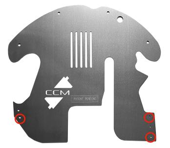
Step 5: The two remaining holes on the front shield will be drilled with a 5/32" drill bit and the security screws will then be installed with a large flathead screwdriver. This will compete the front shield installation
