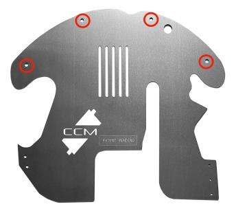
STEP 4: After the front four rivets are installed, use the pre-drilled holes in the shield as guides to drill the remaining holes into the frame of the vehicle. On the driver side drill any two of the three holes with a 3/16" drill bit and install two of the remaining rivets. On the passenger side drill a single 3/16" hole and install one rivet.
