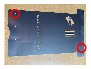
Step 2 - Once the Cat Security<sup>TM</sup> shield is stable, proceed to drill out the inner holes for the rivets. Install the rivets using the 1/2" rivet gun.
