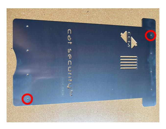
$Step \ 2 \ - \ Once the \ \Box at \ Security \ \ \ shield is stable, proceed to drill out the inner holes for the rivets. Install the rivets using the 1/2" rivet gun.$
