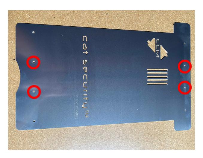
Step 3 - Install the security screws in the corners of the Cat Security shield. You can use the self-tapping screws to make the holes for the security screws, if you do not have a 5/16" drill bit. Install security screws and you are done.
