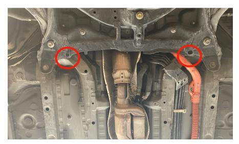
Before tightening the security bolts firmly down, ensure the support brace is pulled back as far as possible. The support brace and the subframe need to be as flush as possible. The installed brace should look like the picture below.
