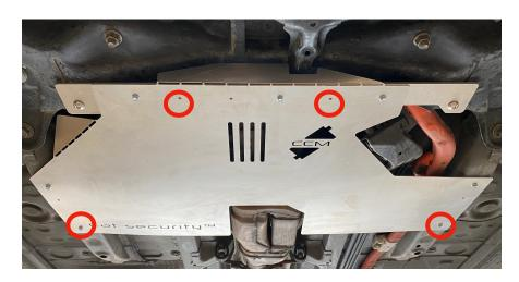
$Step\ 3$  - Using a 3/16" drill bit, drill holes in the front support brace as shown and install the (2) 3/16" long rivets. Drill out the sides as show and install the remaining (4) rivets.
