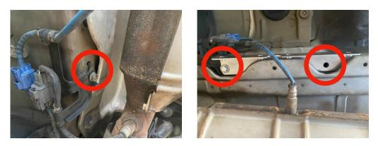
STEP 1:- <u>All Wheel Drive</u> has two bolt holes on the drivers rail. This is for the AWD driveline brace. Remove the bolt and install the rail. bend the driveshaft loop strap brace to ensure ample clearance around the driveshaft. Reuse the existing factory bolt.
