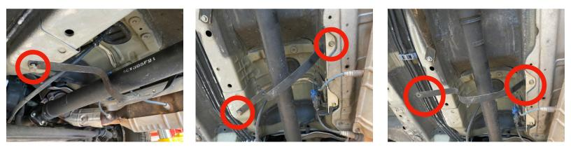
STEP 2: Install Passenger Side Mounting Rail (passenger side, rail with 3 mounting holes) Install the passenger mounting rail going between the heat shield and body. The front flange bolt is supplied, reuse the factory middle bolt, then drill the hole for the 3/16" rivet and install it. Ensure the other two bolts are tight and this step is complete.
