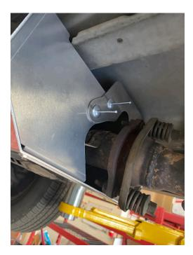
\*Cat Daddy Pro Tip\*: For added protection, use silicone in the head of the security torx bolts to make it harder to remove.
