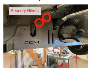
Step 3 - Install Mid shield TAB
