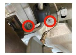
Install the bottom part of the box and temporarily install (DO NOT CRIMP YET) rivets to align the box bolt holes.
