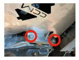
Step 2 - Installing the mid shield.
