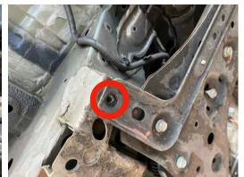
The first image shows the mid shield installed without security hardware. It is CRITICAL that you open the gap between the subframe and frame rail in order to slide the shield in. Use a prybar or large flat screw driver pry in-between. Area is circled in the first picture.
