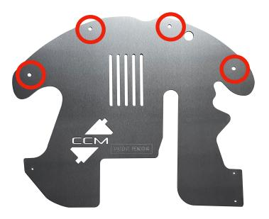
STEP 3: Locate the  $\frac{1}{4}$ " rivets (the larger of the two included in hardware kit) make sure the front four holes line up properly then using a heavy-duty  $\frac{1}{2}$ " rivet gun insert and install the front 4 rivets into the existing holes.
