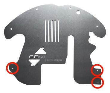
Drill the remaining 3/16" holes. Using the spacers and longer rivets, install and check for clearance around the exhaust.
