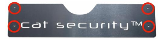
Drill out the 4 holes in the rear shield using the holes as guides. Install the remaining rivets and check for clearance.
