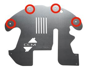
STEP 3: Locate the ¼" rivets (the larger of the two included in hardware kit) make sure the front four holes line up properly then using a heavy-duty ½" rivet gun insert and install the front 4 rivets into the existing holes.
