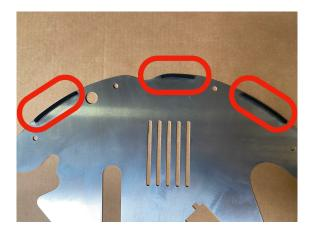
With the radius of the front shield facing towards the front of the vehicle slip the shield into place aligning the front four holes with the factory clip holes that we removed the plastic clips from in step one.
