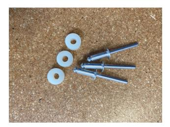
Once the front four rivets are installed you can then use the predrilled holes in the plate as a guide to drill your holes on the vehicle.
